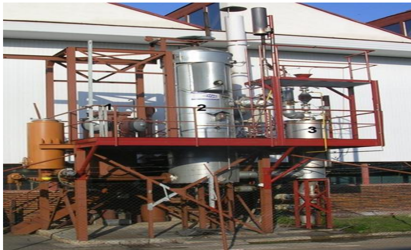
Figure 1 : Atmospheric fluidized bed gasifier Biofluid 100
