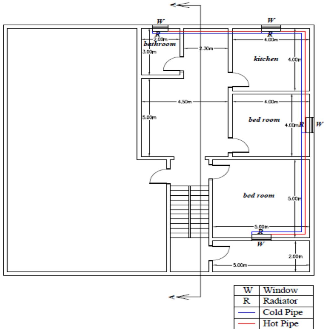
Fig. 11.24 Scheme of Large House first floor
