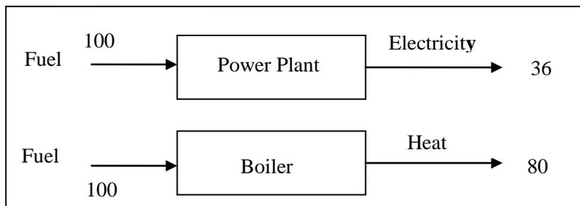
**Fig. 8.3 Separate production of electricity and heat [23]**
