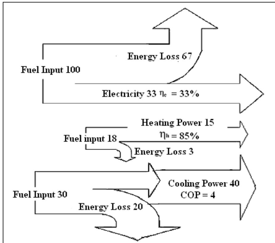
Fig. 9.8 Energy flow of traditional supply mode [27]
