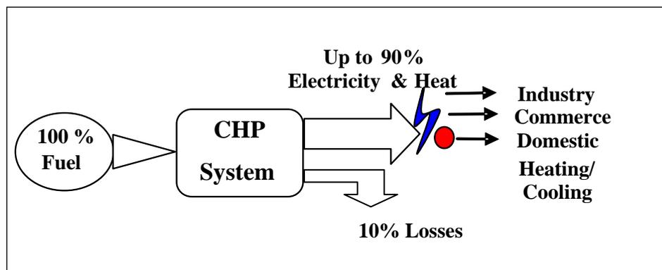
**Fig. 8.1 Schematic diagram of Cogeneration (CHP) [20]**
