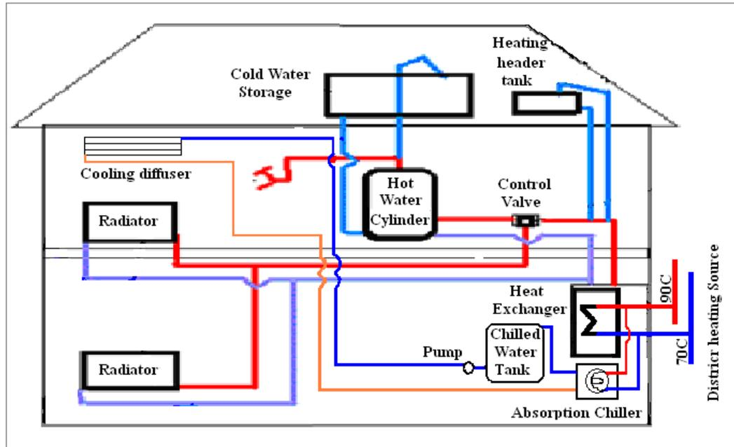
Fig. 11.6 Heating /cooling system for typical house
