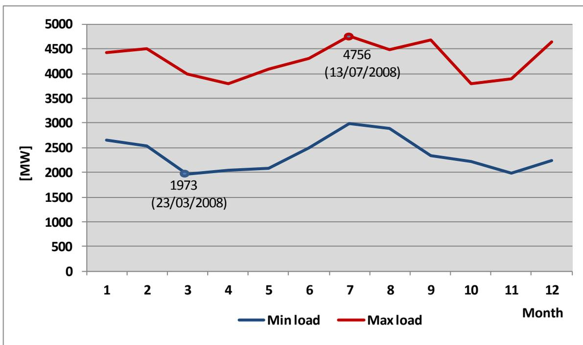
Fig. 4.18 Maximum and minimum load in 2008
