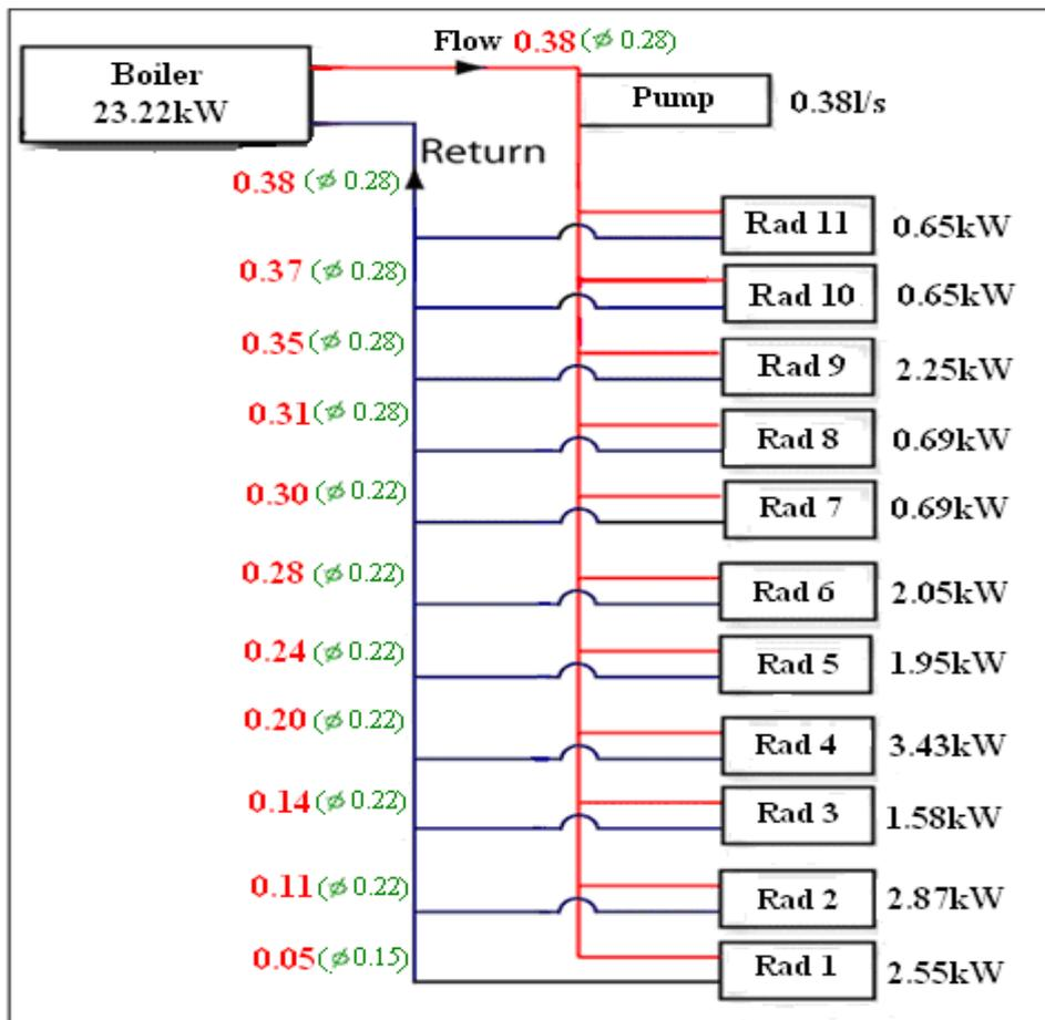
Fig. 11.22 Heating system of medium house
