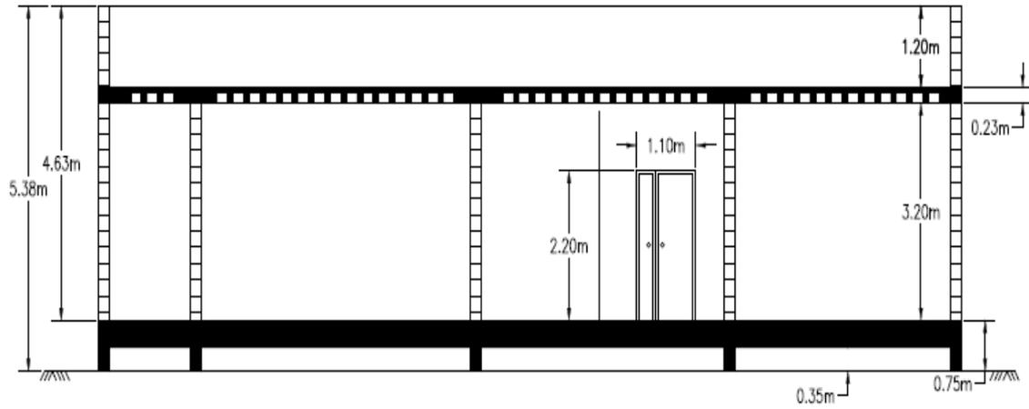
**Fig. 11.19** Cross section A-A of the building
