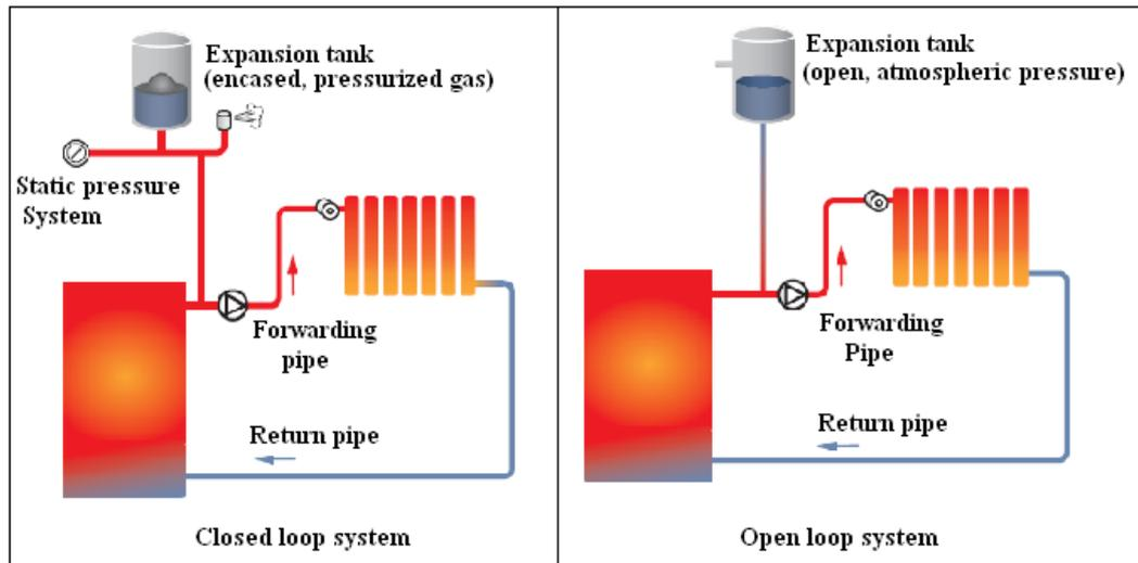
Fig. 11.8 Closed and Open loop systems [43]
