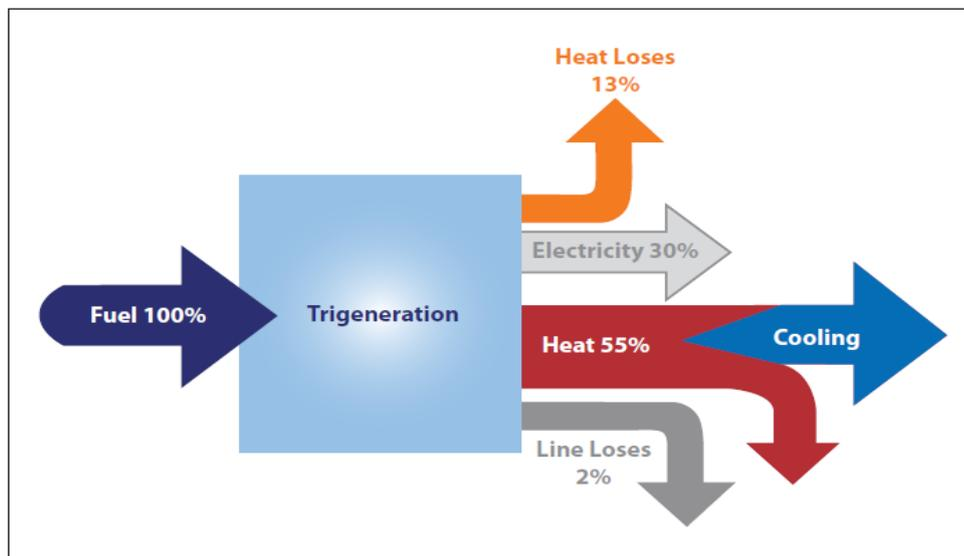
**Fig. 9.1 Schematic diagram of Tri-generation process [24]**
