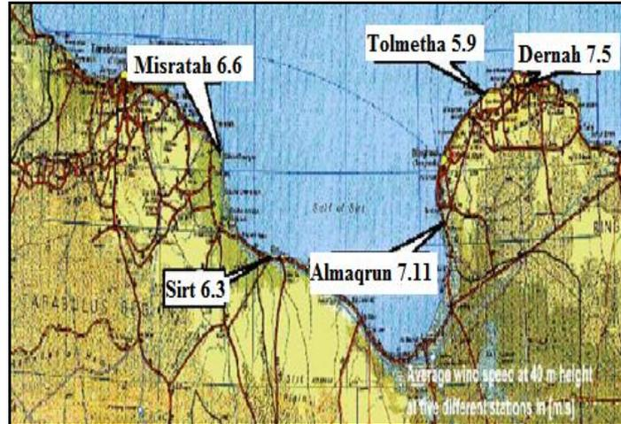
Fig. 4.6 Wind potential for Libyan coast area – average wind speed in m/s [11]
