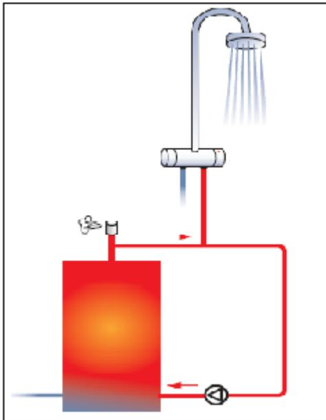
**Fig. 11.10** Hot water system
