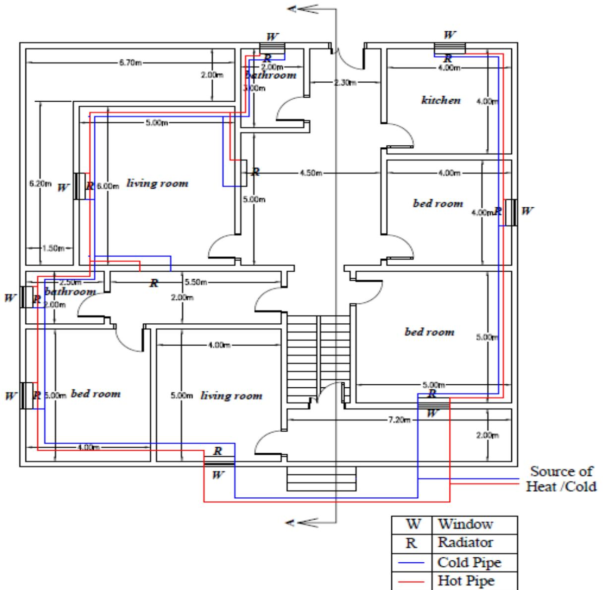
Fig. 11.23 Scheme for large house ground floor
