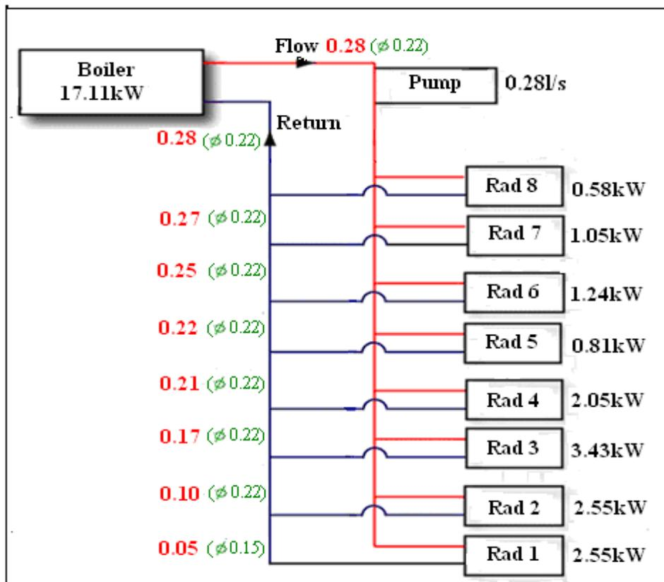
Fig. 11.17 Heating system of small house
