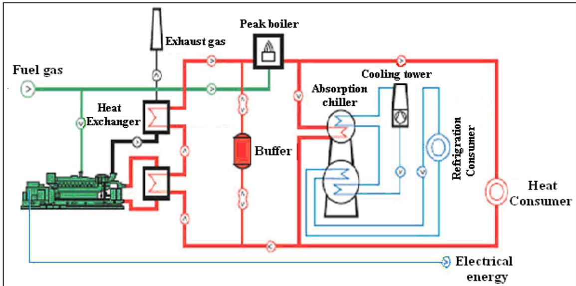
Fig. 9.2 Schematic showing overall tri-generation system configuration [24]
