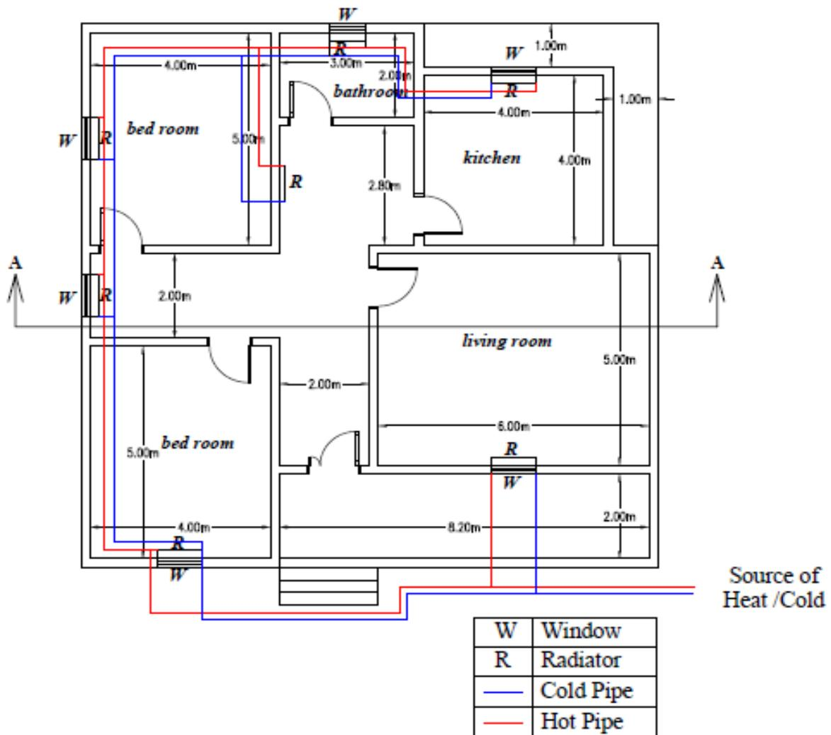
Fig. 11.13 Scheme for small house (Horizontal view)
