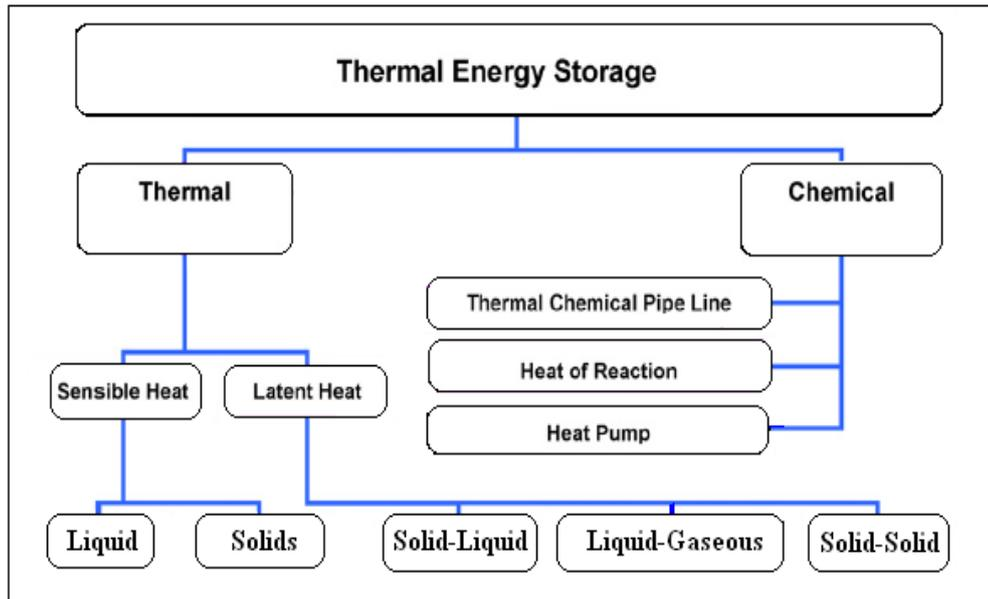
**Fig. 10.4 Different types of thermal energy storage [34]**
