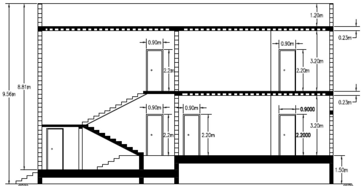
Fig. 11.25 Cross section A-A of the building
