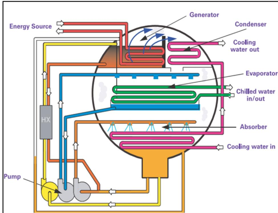
**Fig. 9.4 The principal of an absorption cooling machine**
