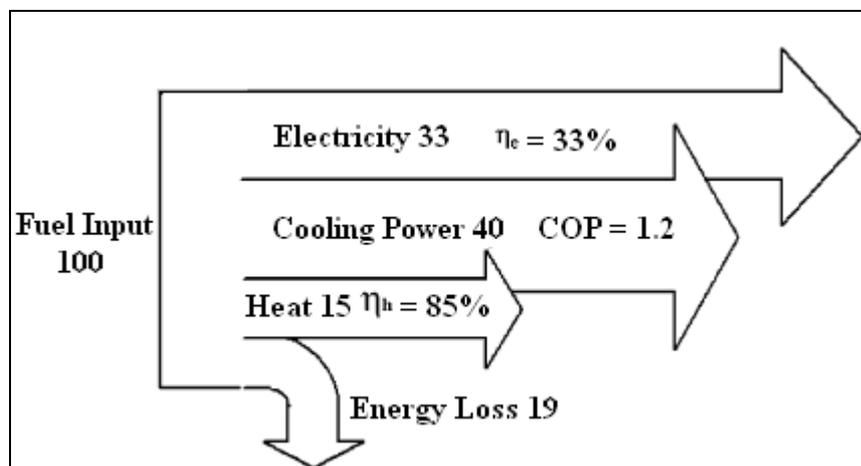
Fig. 9.9 Energy flow of typical CHCP system [27]
