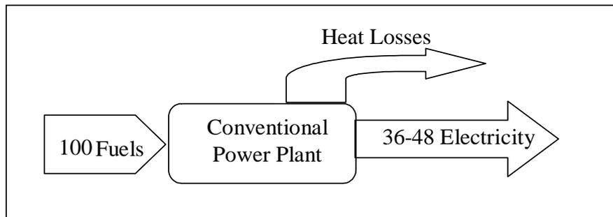
**Fig. 7.2 Simple scheme for conventional power plants**
