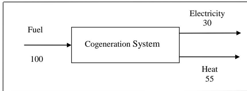
**Fig. 8.4 Cogeneration (CHP) production of electricity and heat [23]**
