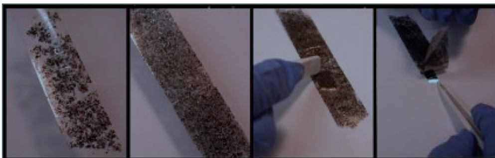
FIGURE 3.12: Exfoliation of graphene using the scotch tape method [36].
