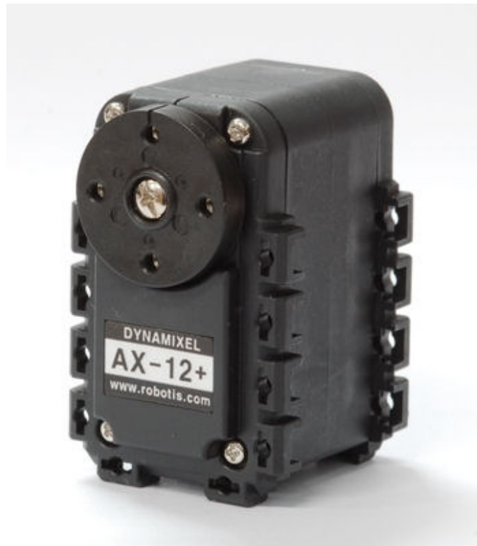
Pic. 9: The AX-12+ servo actuator [5]
