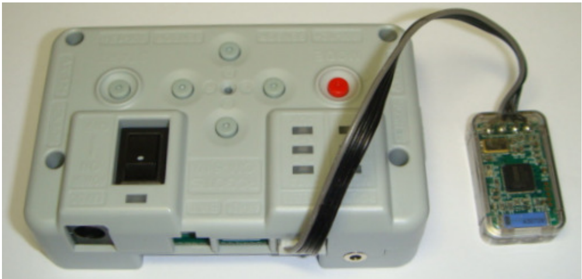
Pic. 18: Zig-110 Wireless Communication Module connected to the CM-510 [4]
