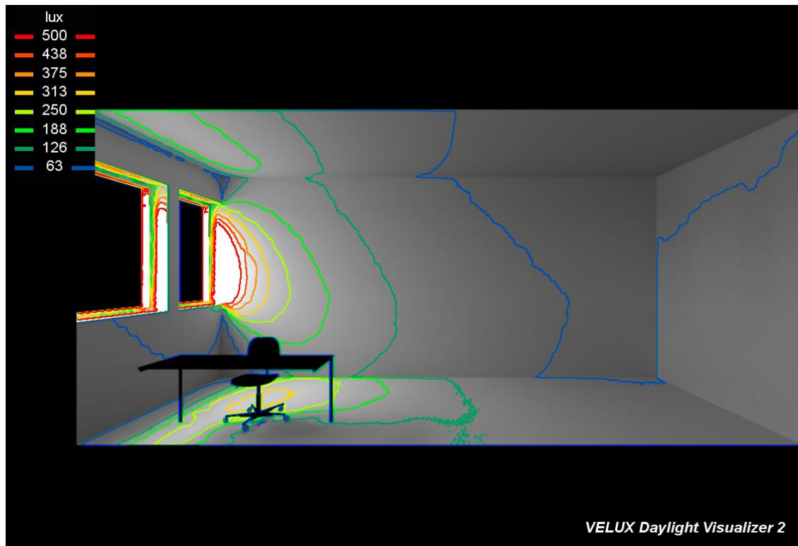
Picture 3 : Illuminance evaluation sectional view (lux) Source: Own work in program VELUX Daylight Visualizer
