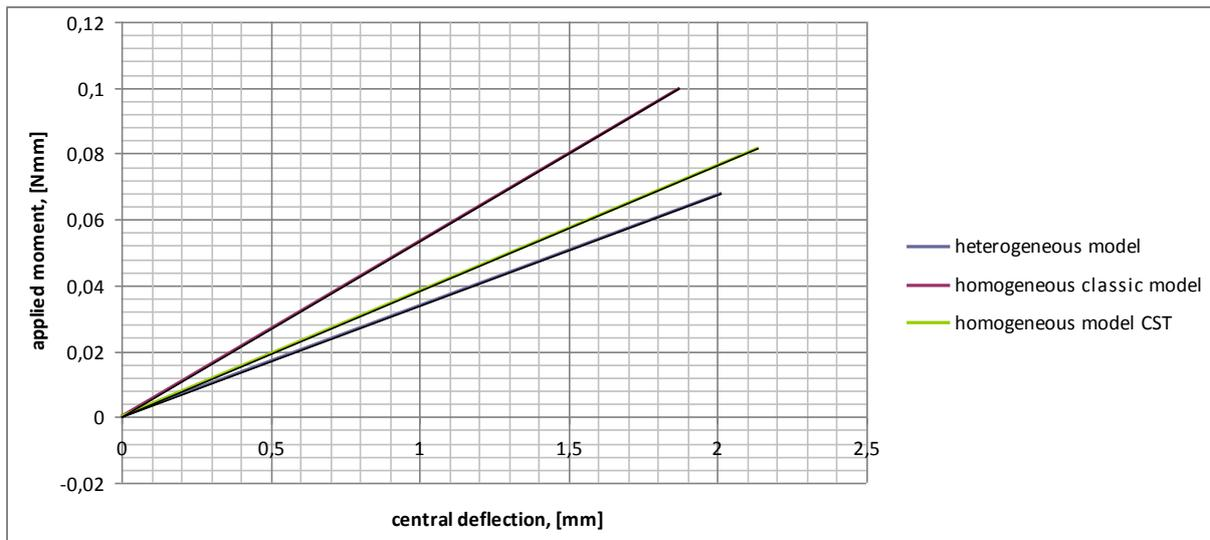
Fig. 5.4. Comparison of FE simulations of 4-point bending using different constitutive models for the case of fibre declination angle of 30 degrees.
