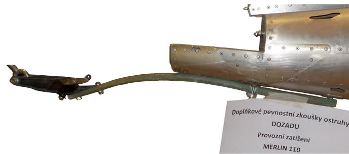
Figure 5.34: Supplementary condition up + aft - limit load.
