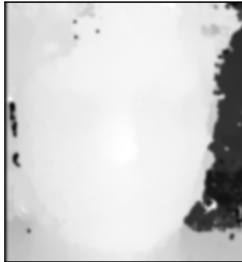
Figure 4.1: Good disparity map. This is how it should look. Smooth surface and no holes.
