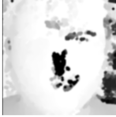
Figure 4.2: This disparity map is not usable, because area with nose and around eyes wasn't reconstructed well. However if you see this, you are on a good way, this probably signifies problem with illumination, but the reconstruction algorithm works well.
