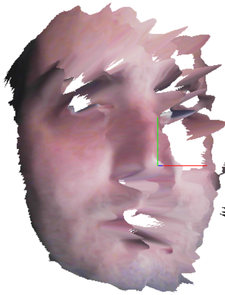
Figure 6.3: Webcam model with errors in disparity map, manual method.
