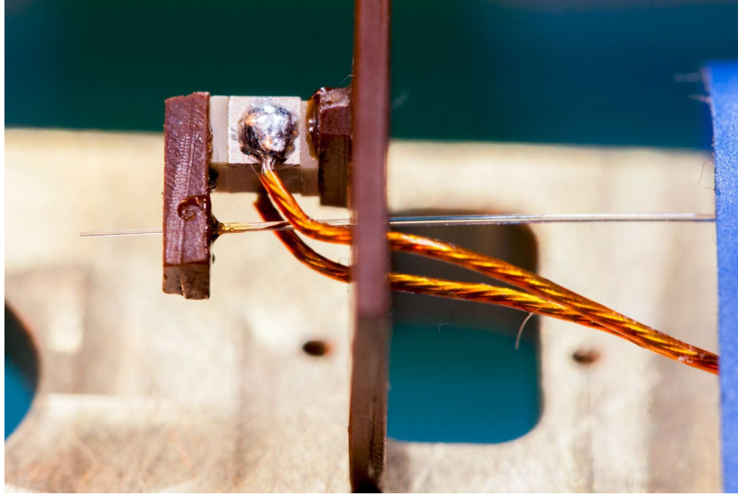
Fig. 4.14: A picture of the interferometric sample holder assembly. We can see there the piezoelectric crystal glued to the movable platform from one side and the fiber tip holder from the other. All parts are glued together with low temperature varnish.
