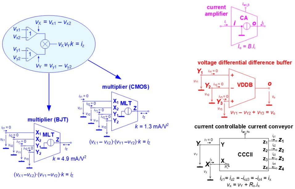
Fig. 2.1 Symbols of active elements/cells in fabricated IC (0.35  $\mu\text{m}$  I3T ON Semiconductor process) and their fundamental principle expressed by inter-terminal relations
