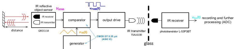
Fig. 5.5 Block concept of system proposed for measuring distance and signal distribution
