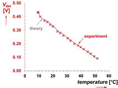
Fig. 5.10 Dependence of detected/received voltage on temperature
