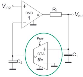
Fig. 3.1 Circuit topology of band-pass filter designed for experiments with center frequency tunability range
