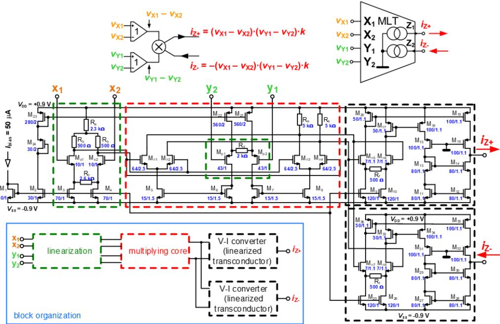
Fig. 2.4 Operational principle, symbol and internal topology of double output CMOS MLT designed and fabricated using  $0.18\text{ }\mu\text{m}$  TSMC process
