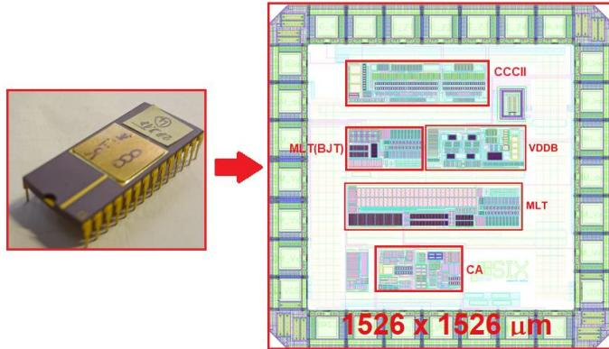
Fig. 2.3 Package and top-layout of fabricated IC including five different active elements/cells
