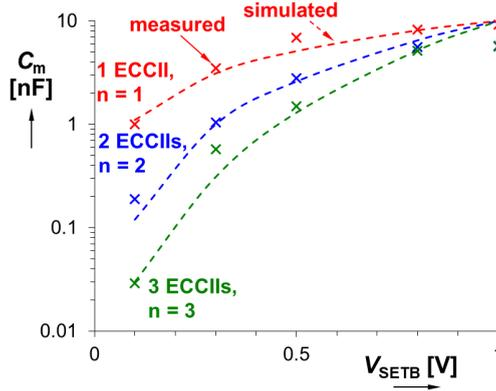
Fig. 3.8 Dependence of  $C_m$  on current gain  $B$  ( $V_{SETB}$ ) for a variation of the number of ECCII in the structure ( $n = 1, 2$  and  $3$ )
