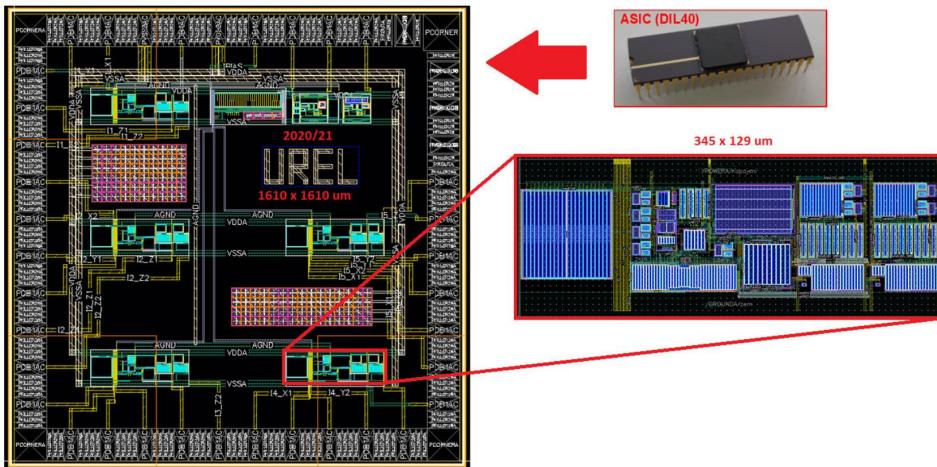
Fig. 2.5 Package, top-layout and cell layout of MLT ( $0.18\text{ }\mu\text{m}$  TSMC process)
