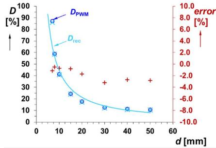
Fig. 5.7 Comparison of transmitted and received duty cycle of square waves in dependence on measured distance
