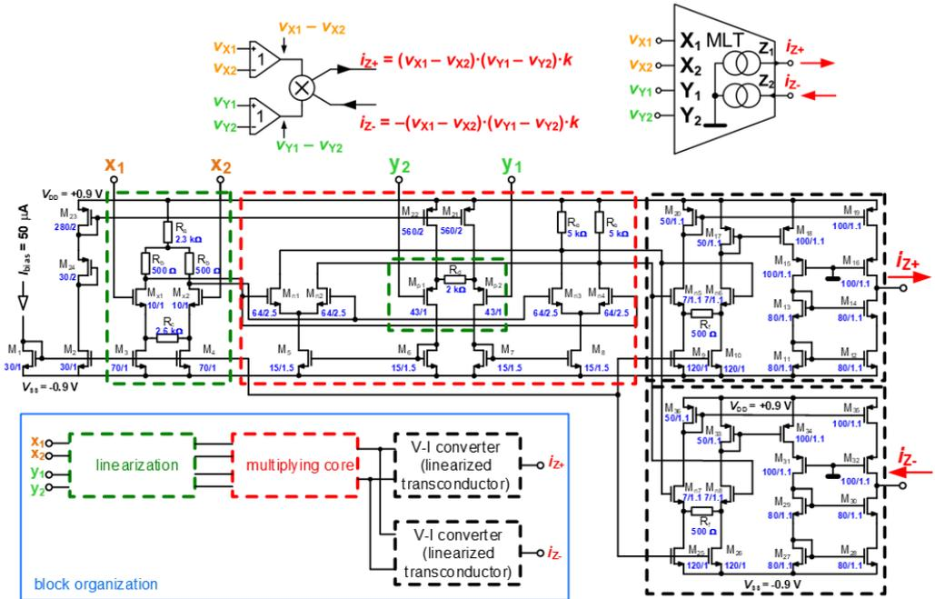
Fig. 2.4 Operational principle, symbol and internal topology of double output CMOS MLT designed and fabricated using 0.18  $\mu\text{m}$  TSMC process
