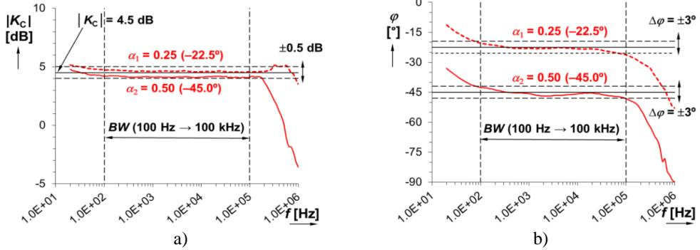
Fig. 4.4 The frequency response of CPB: a) magnitude, b) phase responses
