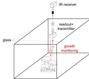
Fig. 5.4 Illustration of measurement of height of plants and distribution of signal from a closed agricultural reservoir for cultivation
