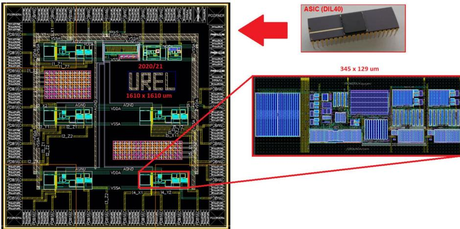
Fig. 2.5 Package, top-layout and cell layout of MLT (0.18  $\mu\text{m}$  TSMC process)
