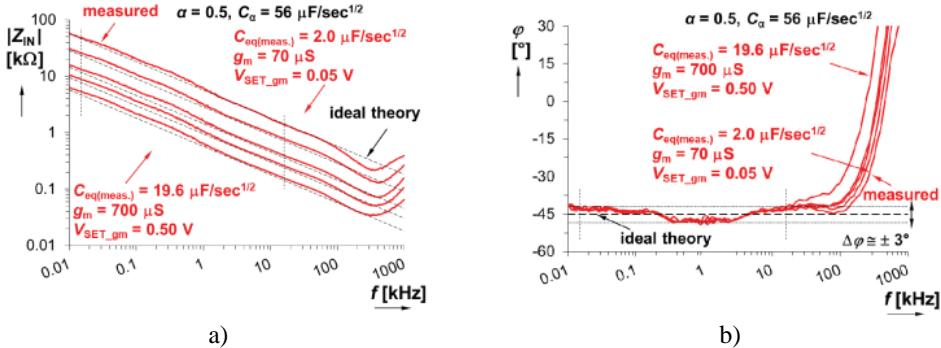
Fig. 4.6 Example of operation and electronic adjustability of equivalent capacity of a capacitance multiplier: a) magnitude responses, b) phase responses.
