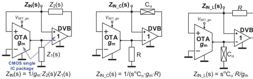
Fig. 4.5 General topology (left) for a fractional-order capacitance multiplier (middle) and impedance inverter generating synthetic inductance (right).
