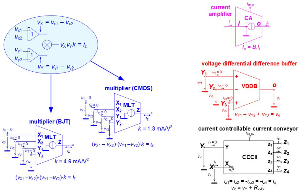
Fig. 2.1 Symbols of active elements/cells in fabricated IC (0.35  $\mu$ m I3T ON Semiconductor process) and their fundamental principle expressed by inter-terminal relations
