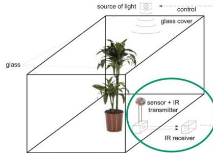
Fig. 5.2 Example of application in transmission of measured illuminance from a closed agricultural reservoir for cultivation of plants
