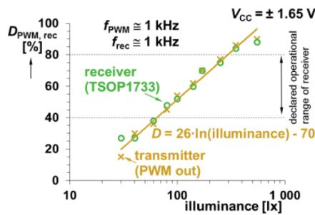
Fig. 5.3 Example of transmitted and received duty cycle in dependence on illuminance
