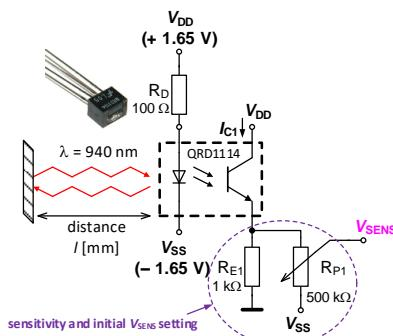
Fig. 5.6 Principle of the IR reflective sensor
