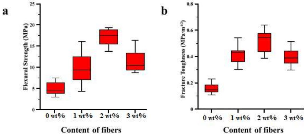
**Figure 9: a) Flexural strength and b) fracture toughness of the geopolymer matrix composite.**
