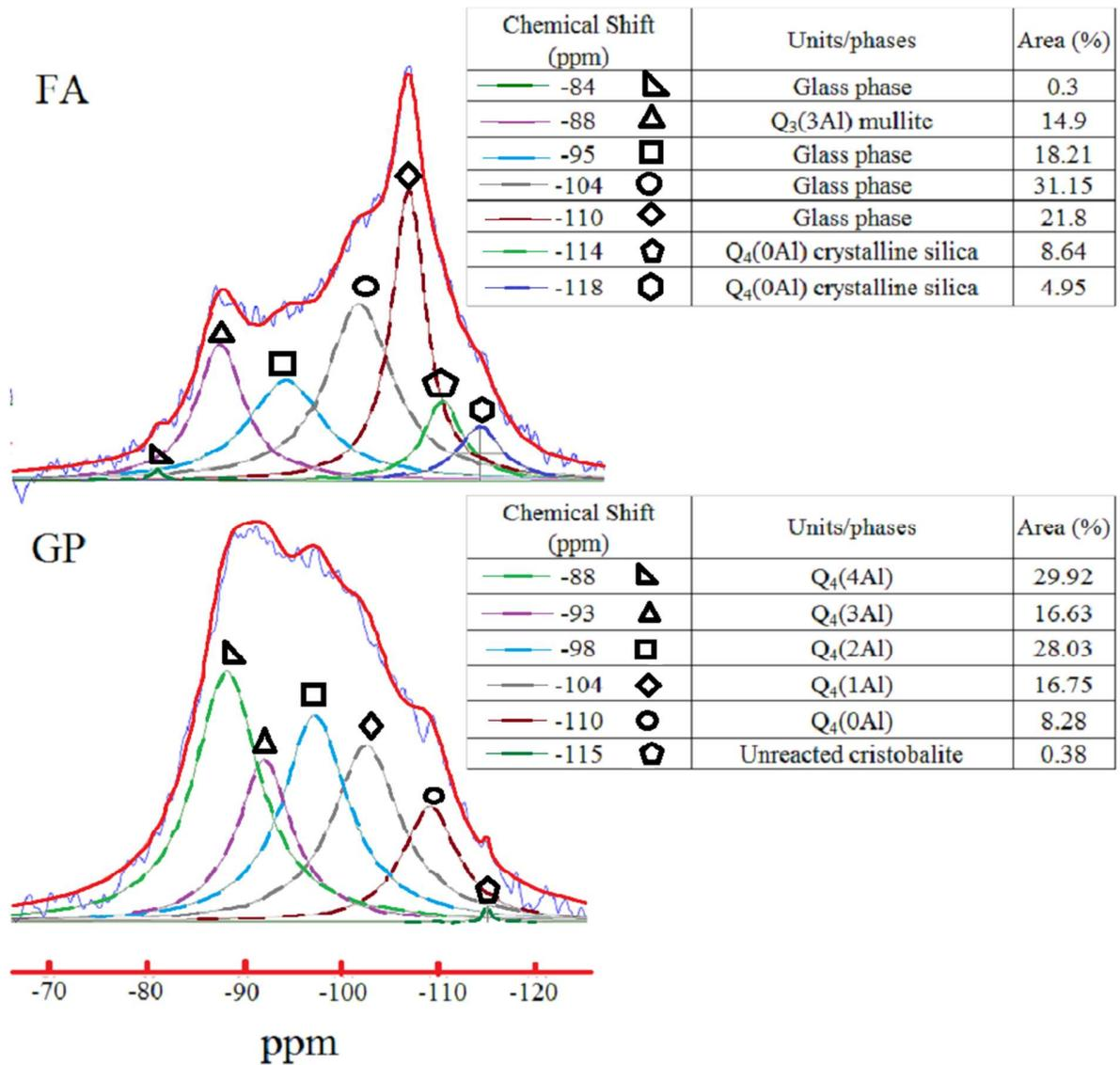
**Figure 6:** <sup>29</sup>Si magic angle spinning nuclear magnetic resonance spectra of fly ash and geopolymer sample Mix-1.
