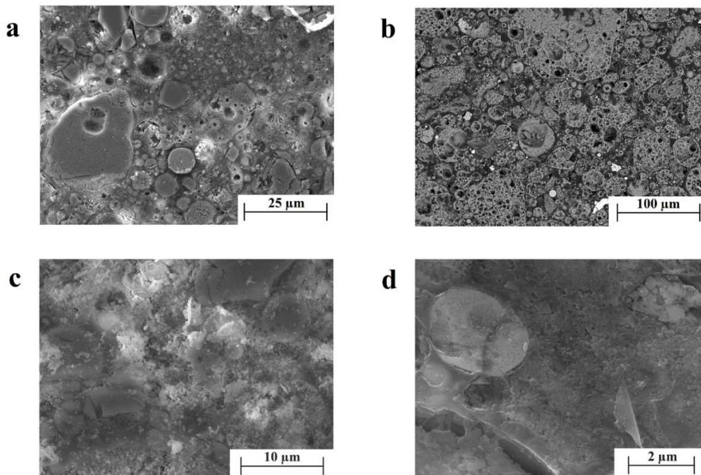
**Figure 10: Scanning electron microscopy of fly ash densified in according to the hydro-pressure sintering process under 500 MPa for 5 minutes in a) water, b) 3M NaOH solution, c) 5M NaOH solution and d) a detail of the crystals of the sample processed in water.**
