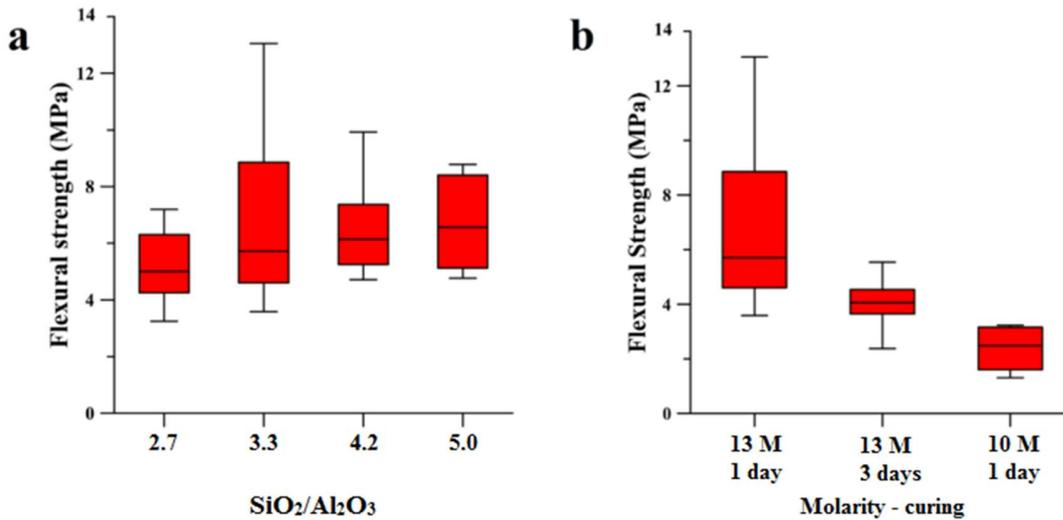
**Figure 8: Flexural strength of geopolymer samples in terms of (a) silica-to-alumina ratio of the mixtures from Mix-1 to Mix-4 (2.7, 3.3, 4.2, 5.0 respectively) and (b) molarity of the activator and curing time used for Mix-2 (13 M for 1 day), Mix-5 (13 M for 3 days) and Mix-6 (10 M for 1 day).**
