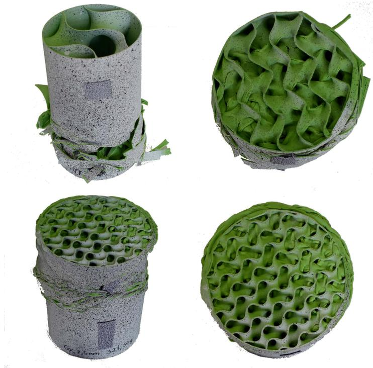
**Obrázek 6.1:** Sample realizations of cylinder compression tests with 3 scales of 3D gyroid infill. Photographed by the author in 2018.
