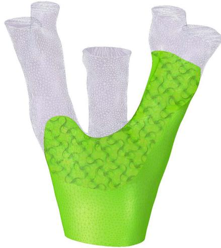
**Obrázek 3.1:** Detail of a branching structure and 3D infill (gyroid). Figure by author.
