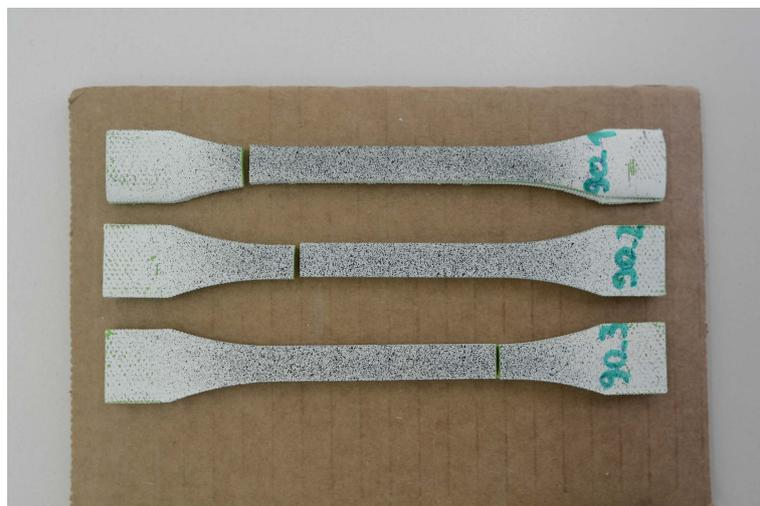
**Obrázek 6.2:** Three realizations of ISO dogbone specimens sliced according to DB 90 after the tensile test. Photographed by the author in 2018.
