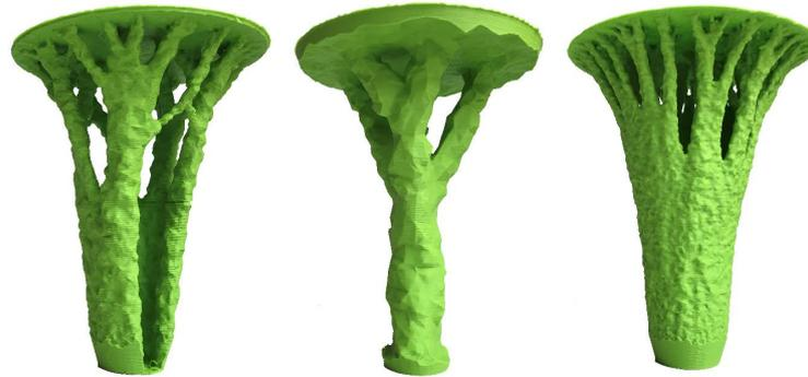
**Obrázek 2.2:** Printouts of topology optimization results and fractal principle: element size governs the overall shape. Photographed by author in 2018.
