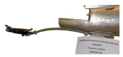
Figure 4.14: Supplementary condition up + aft - limit load.
