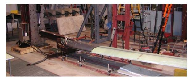
Figure 4.1: Layout of X06 wing segment fatigue test. Archive of IAE.
