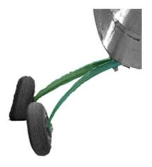
Figure 2.4: Composed picture of main landing gear during drop test. Un-deformed and maximum deformation. Courtesy of TechProAviation, s.r.o.
