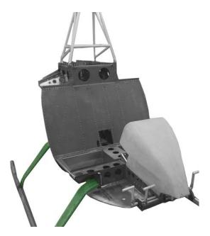
Figure 5.3: Main landing gear (in green) of a helicopter. Courtesy of TechProAviation, s.r.o.
