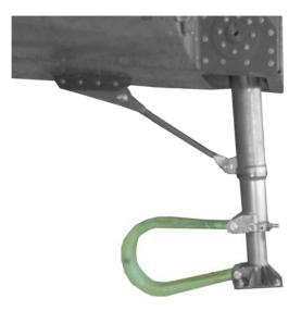
Figure 5.1: Nose gear spring (in green) on Merlin 105 airplane. Courtesy of TechProAviation, s.r.o.
