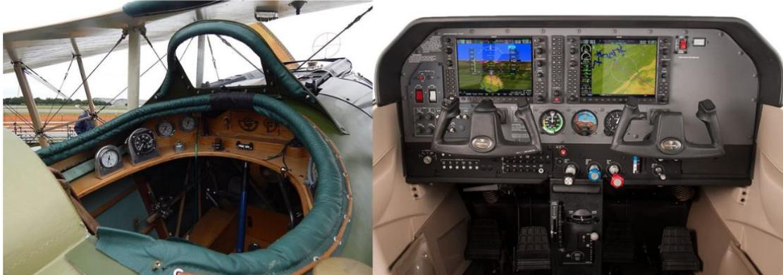
**Figure 1** Comparison of two aircraft cockpits a century apart. Left side is SPAD XIII from 1918, the right side is Cessna 182 Skylane from 2010 [3]
