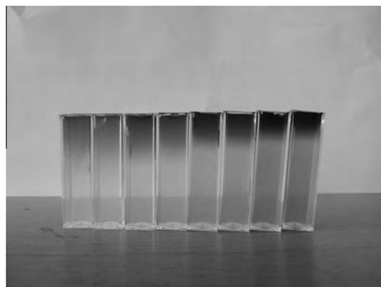
Fig. 5. Picture of the gel samples after 24 h of diffusion of Methylene Blue at 30 °C (four duplicates from left to right: 0 wt.%, 0.002 wt.%, 0.005 wt.% and 0.010 wt.% HA in 1 wt.% agarose gel).
