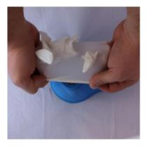
6. Adjust the position of the glove, letting its hem to run (at least approximately) along the halfmask's edge, at a distance of about 2 cm.
