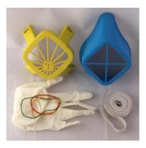
2. Lay the frame (BUTMask\_H1\_Frame.stl) on a desk, with the face-fitting side down.
