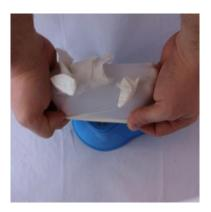
4. Adjust the position of the glove, letting its hem to run (at least approximately) along the edge of the halfmask's edge, at a distance of about 1 cm.
