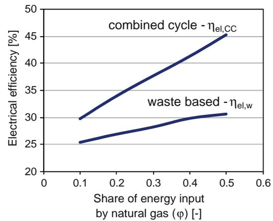
**Fig. 10** Efficiency of integrated system
