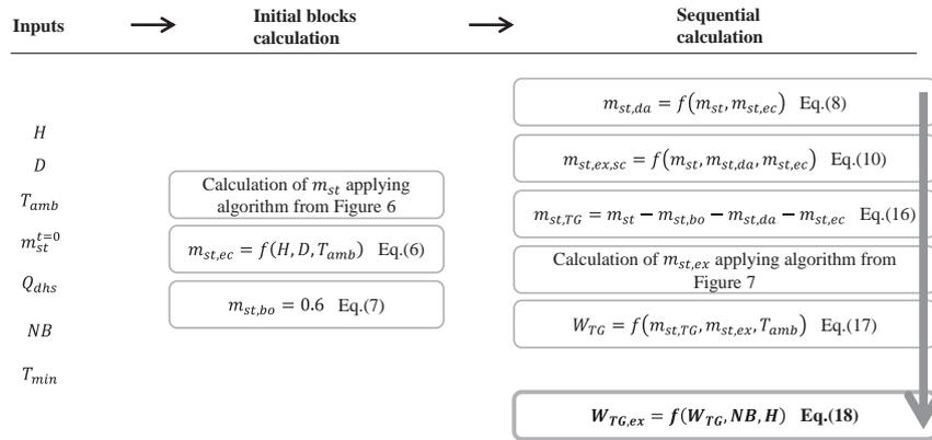
Fig. 8. Sequential calculation of the flow sheet.
