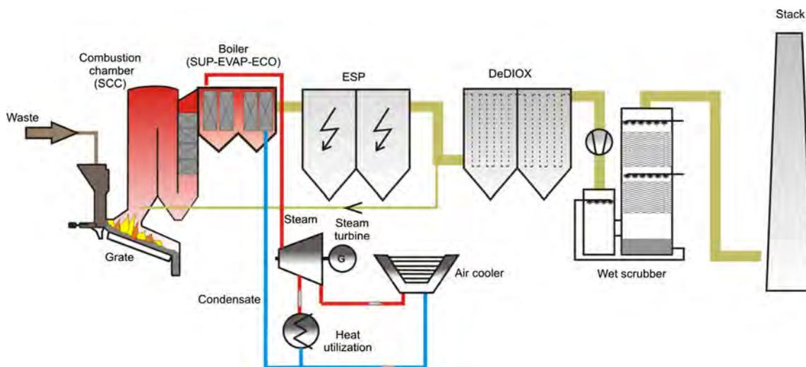
**Fig. 2** Simplified flowsheet of up-to-date technology
