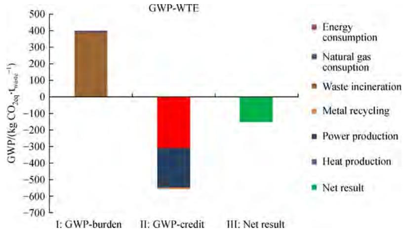
**Fig. 3** WTE: Chart of average annual GWP to 1 t of waste. Capacity =  $100 \text{ kt} \cdot \text{year}^{-1}$ , lower heating value = 8.7, heat export  $4.2 \text{ GJ} \cdot \text{t}^{-1}$ , power export  $0.39 \text{ MWh} \cdot \text{t}^{-1}$
