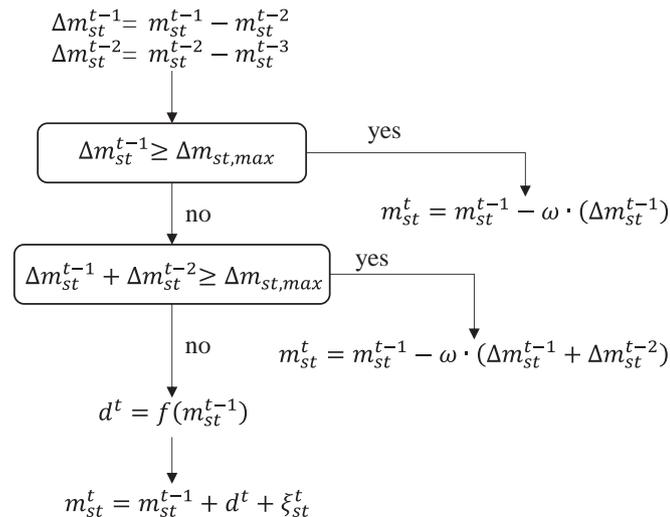
Fig. 6. The algorithm for calculating steam production.
