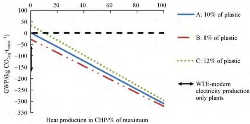
**Fig. 4** WTE: GWP as a function of percentage utilization of heat production. Heat production in CHP = 0% means power-oriented operation; Heat production in CHP = 100% means heat-oriented operation
