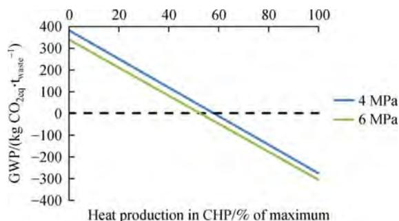
**Fig. 6** Monoblock: GWP as a function of % age utilization of heat production. Heat production in CHP = 0% means power-oriented operation; Heat production in CHP = 100% means heat-oriented operation
