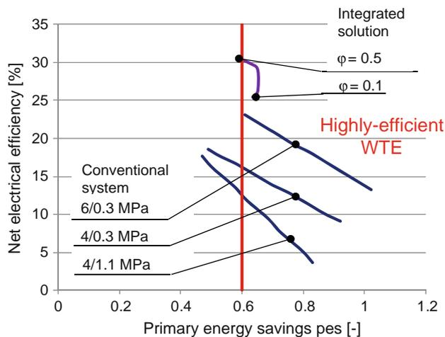
**Fig. 11** Efficiency of waste-based electricity production
