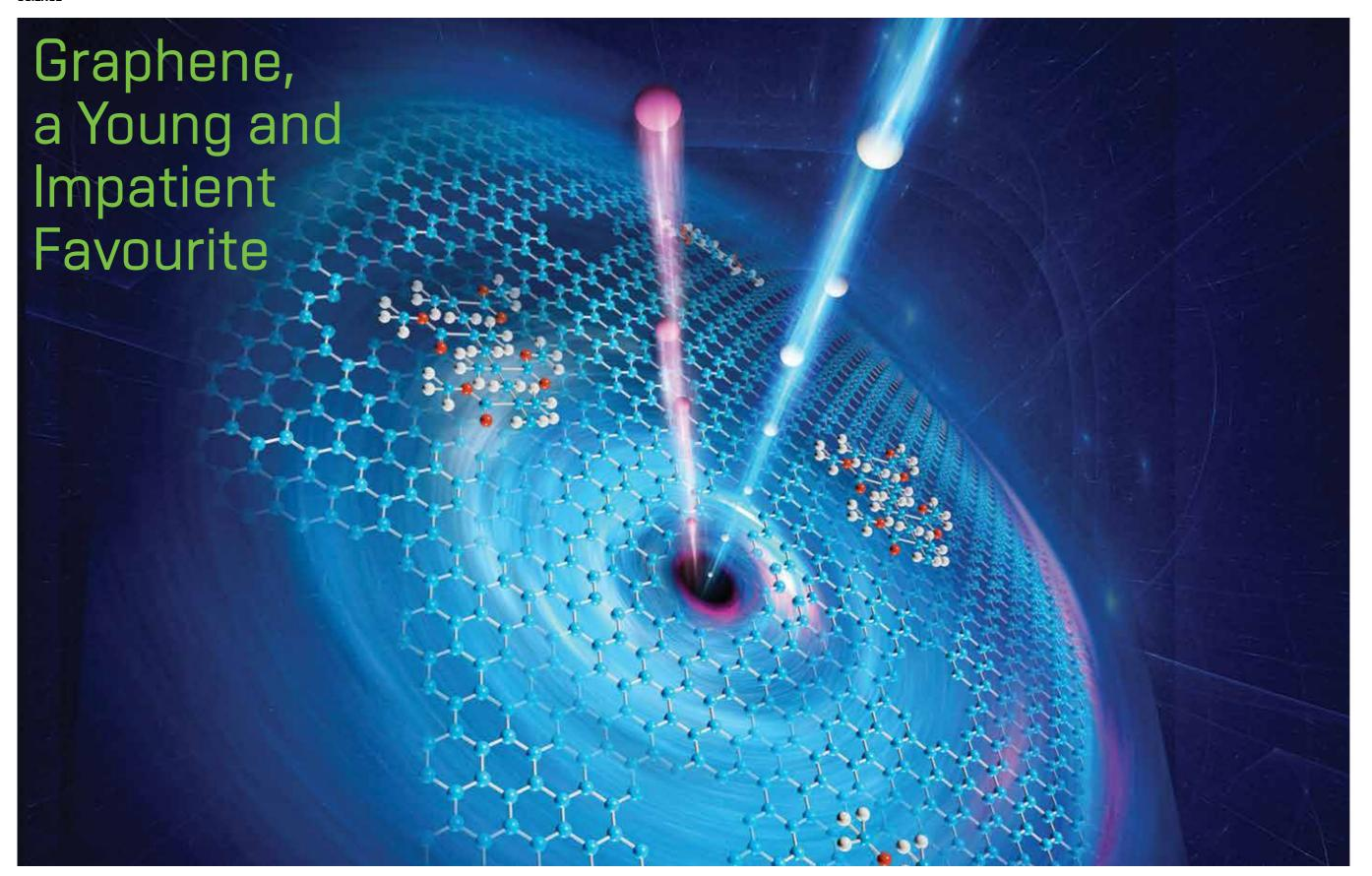
Though looking like a perfect honey-comb, it may be the strongest material in the world. A material of the future for microchips, sensors, solar cells and active membranes, graphene is the most recently described form of carbon; it is very scarce in nature and high quality production is still a problem. As such, the reality of world production still lags behind the theoretical expectations and requirements of industries.
