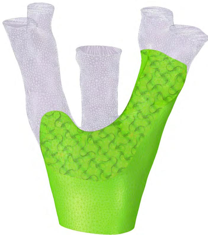
**Figure 6.1:** Detail of a branching structure and 3D infill (gyroid). Figure by author.
