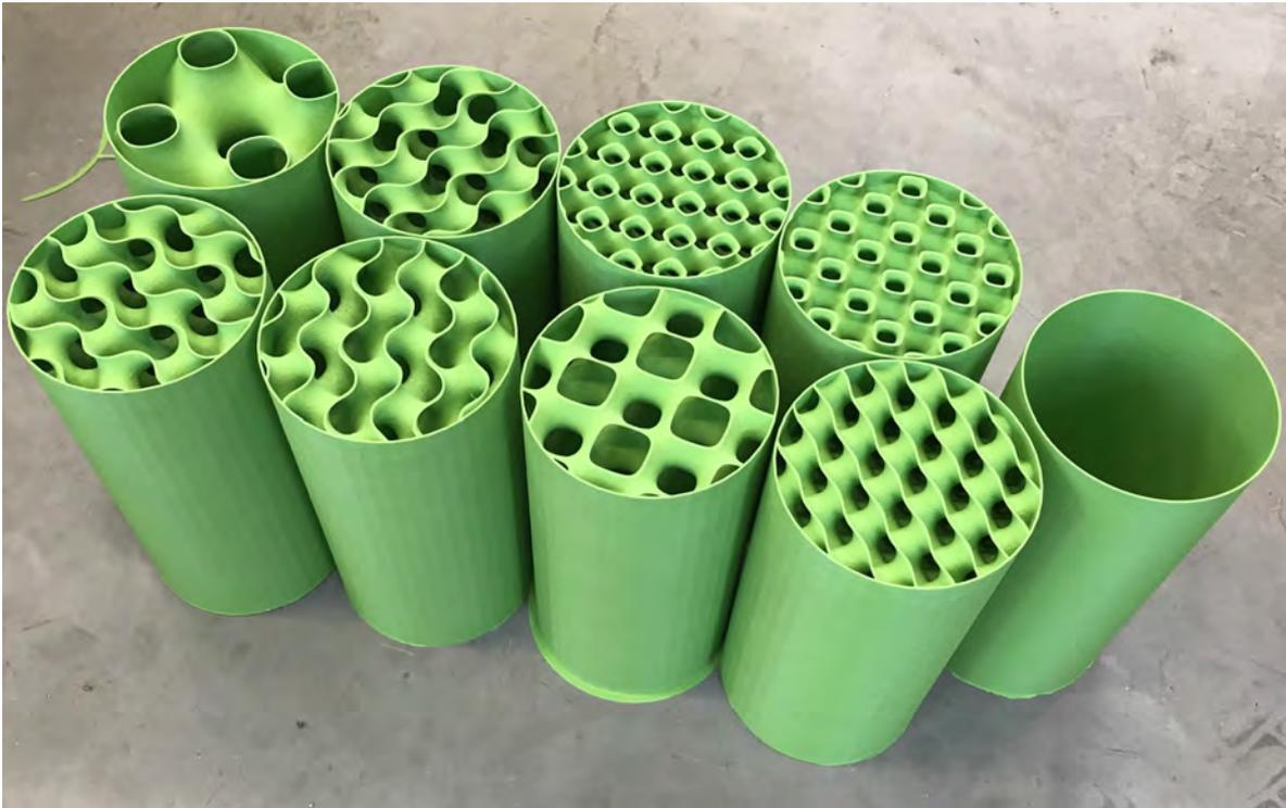
**Figure 9.4:** Sample group of 3D printed specimens from the same filament batch, i.e. same source and storing conditions, in order to eliminate detrimental effects of material degradation and ageing. Photographed by the author in 2018.
