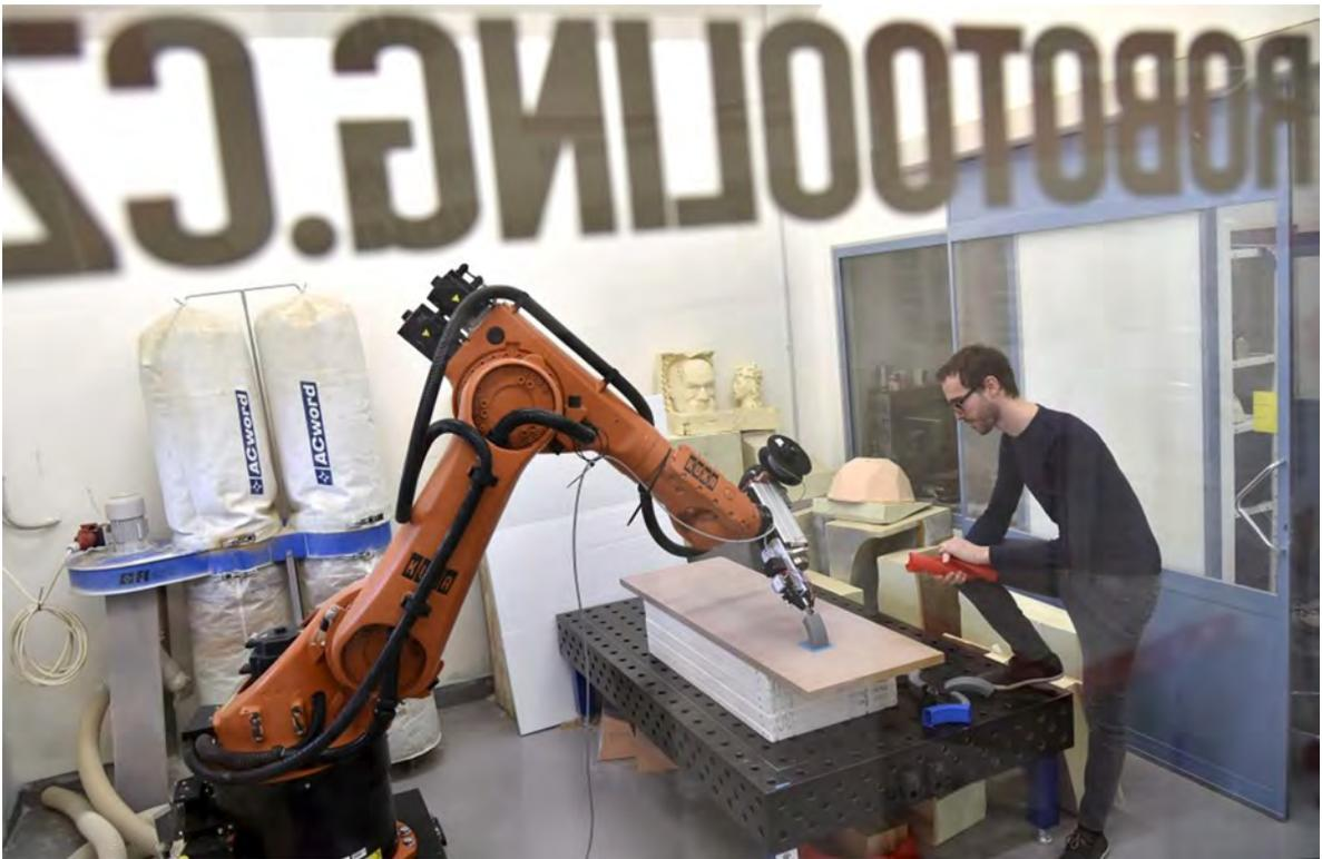
**Figure 4.4:** Kuka six-axis robot and additive manufacturing at StrojLab, which is part the Fab Lab global network. Retrieved from [www.strojlab.cz](http://www.strojlab.cz)
