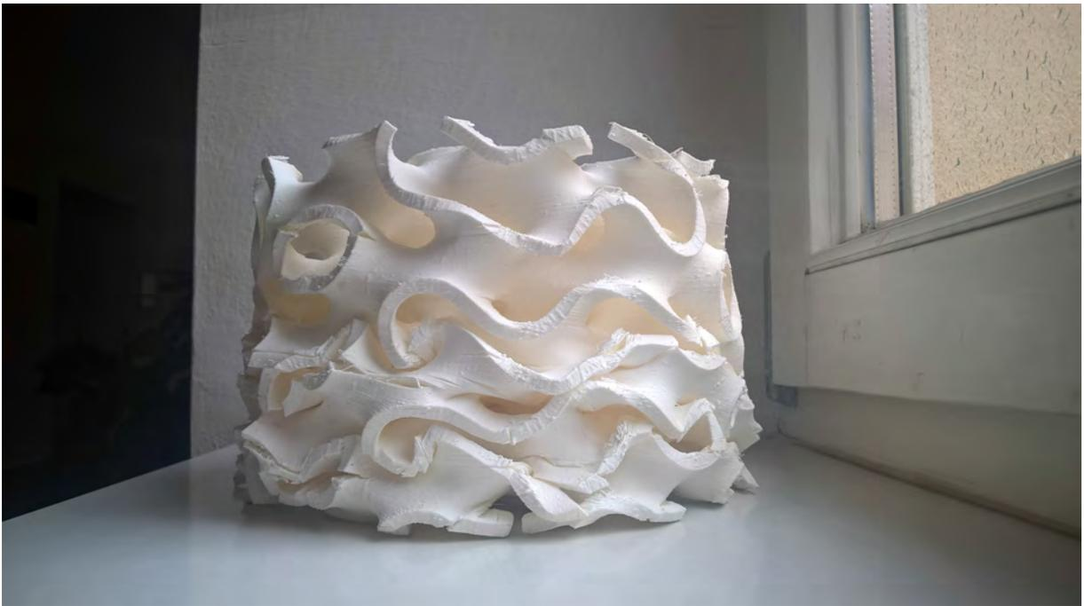
**Figure 7.7:** Gyroid sample printed from PLA after the compression test. Figure by author.
