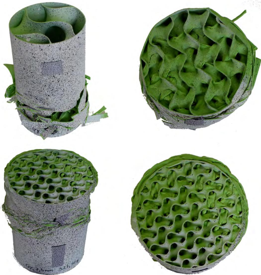
**Figure 9.9:** Sample realizations of cylinder compression tests with 3 scales of 3D gyroid infill. Photographed by the author in 2018.
