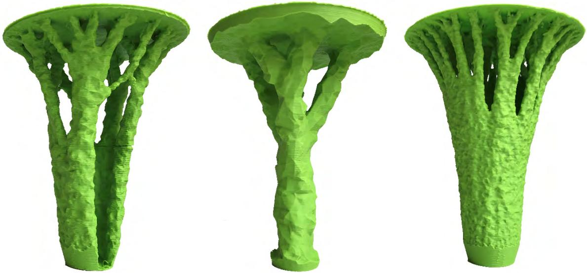
**Figure 5.6:** Printouts of topology optimization results and fractal principle: element size governs the overall shape. Photographed by author in 2018.
