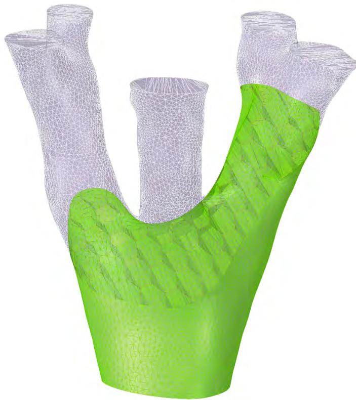
**Figure 6.2:** Detail of a branching structure and 2D infill (hexagonal). Figure by author.
