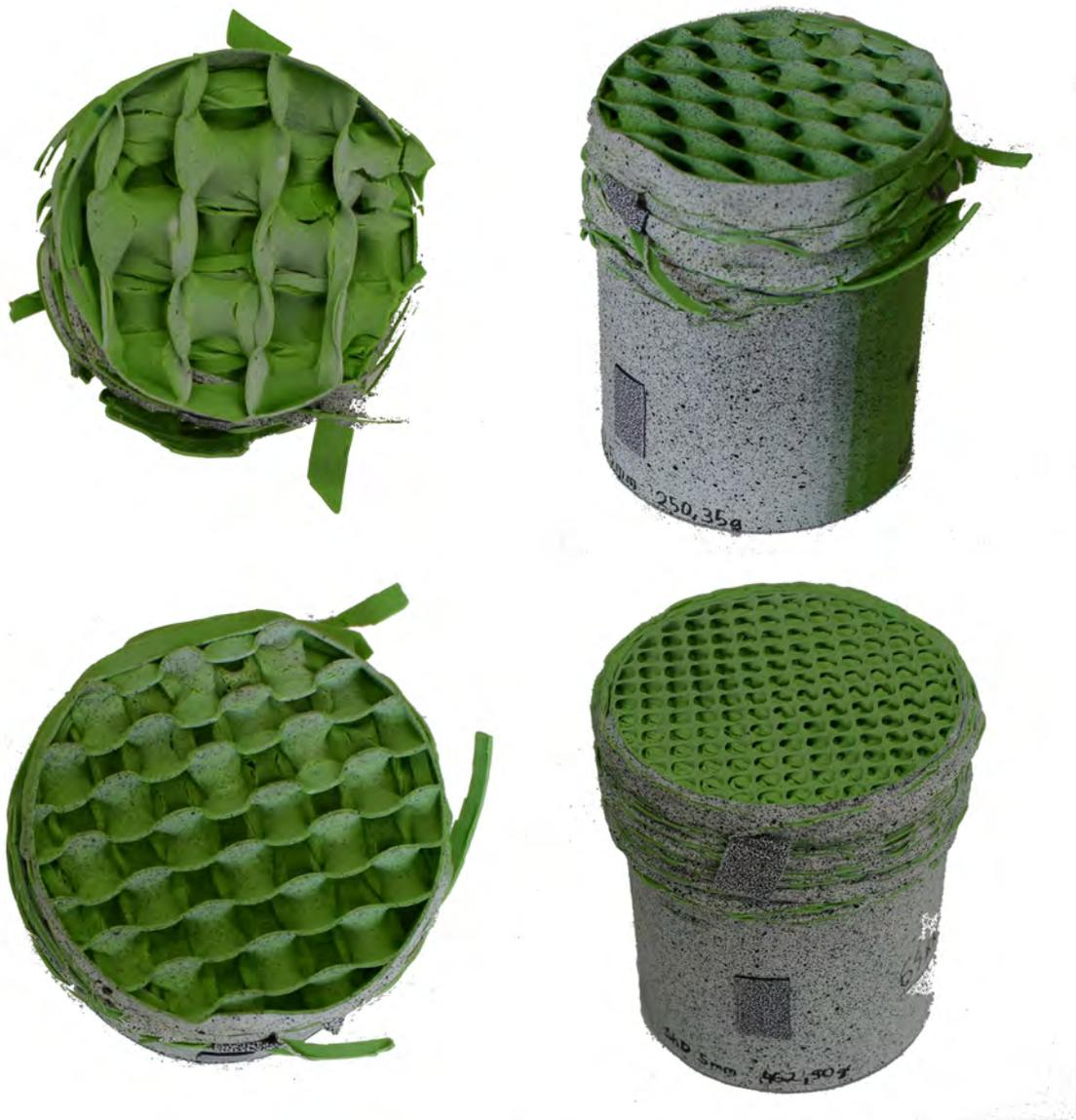
**Figure 9.10:** Sample realizations of cylinder compression tests with 3 scales of 3D Schwarz D infill. Photographed by the author in 2018.
