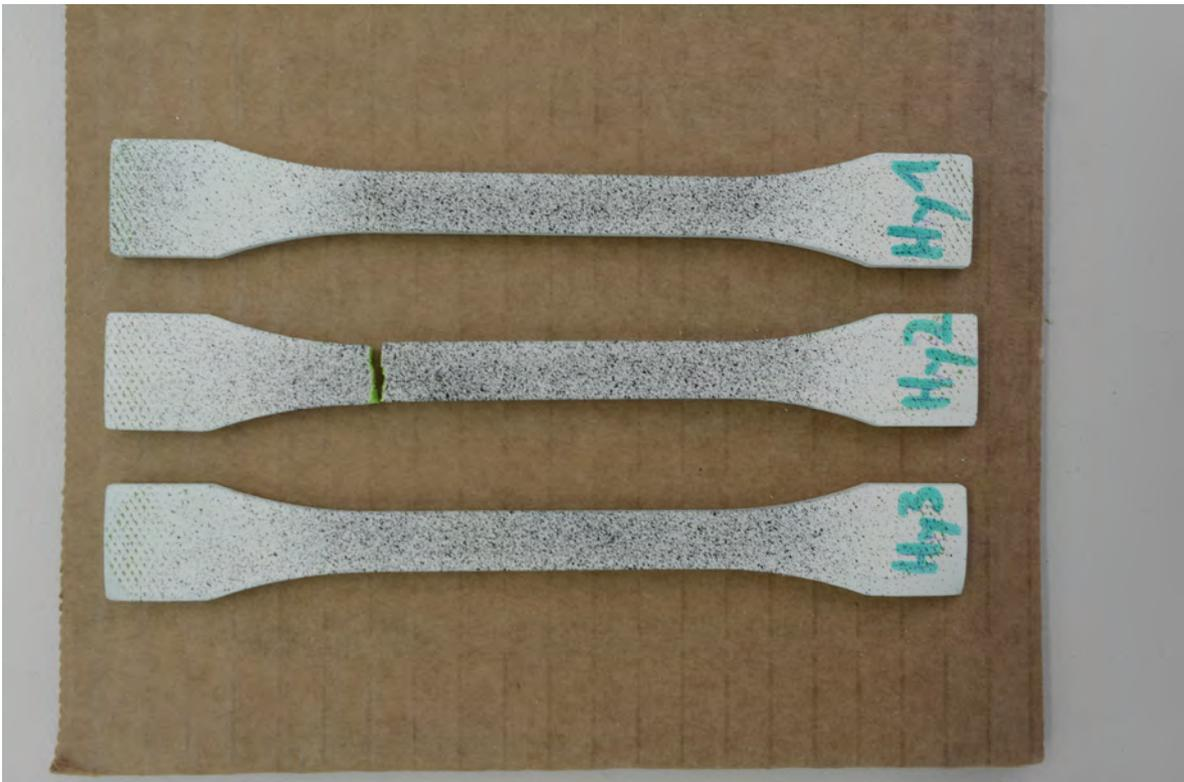
**Figure 9.14:** Three realizations of ISO dogbone specimens sliced according to DB Hy after the tensile test. Photographed by the author in 2018.
