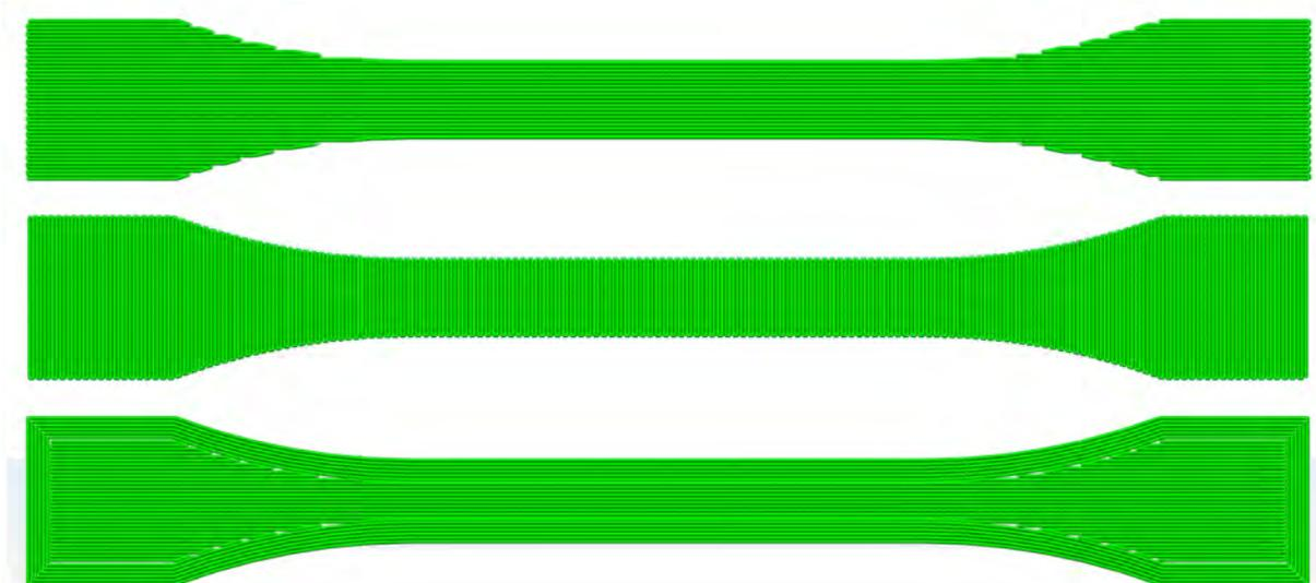
**Figure 9.5:** Different slicing strategies of material characterization based on ISO tensile test specimens (Top: DB 00, center: DB 90 and bottom: DB Hy). Figure by author.
