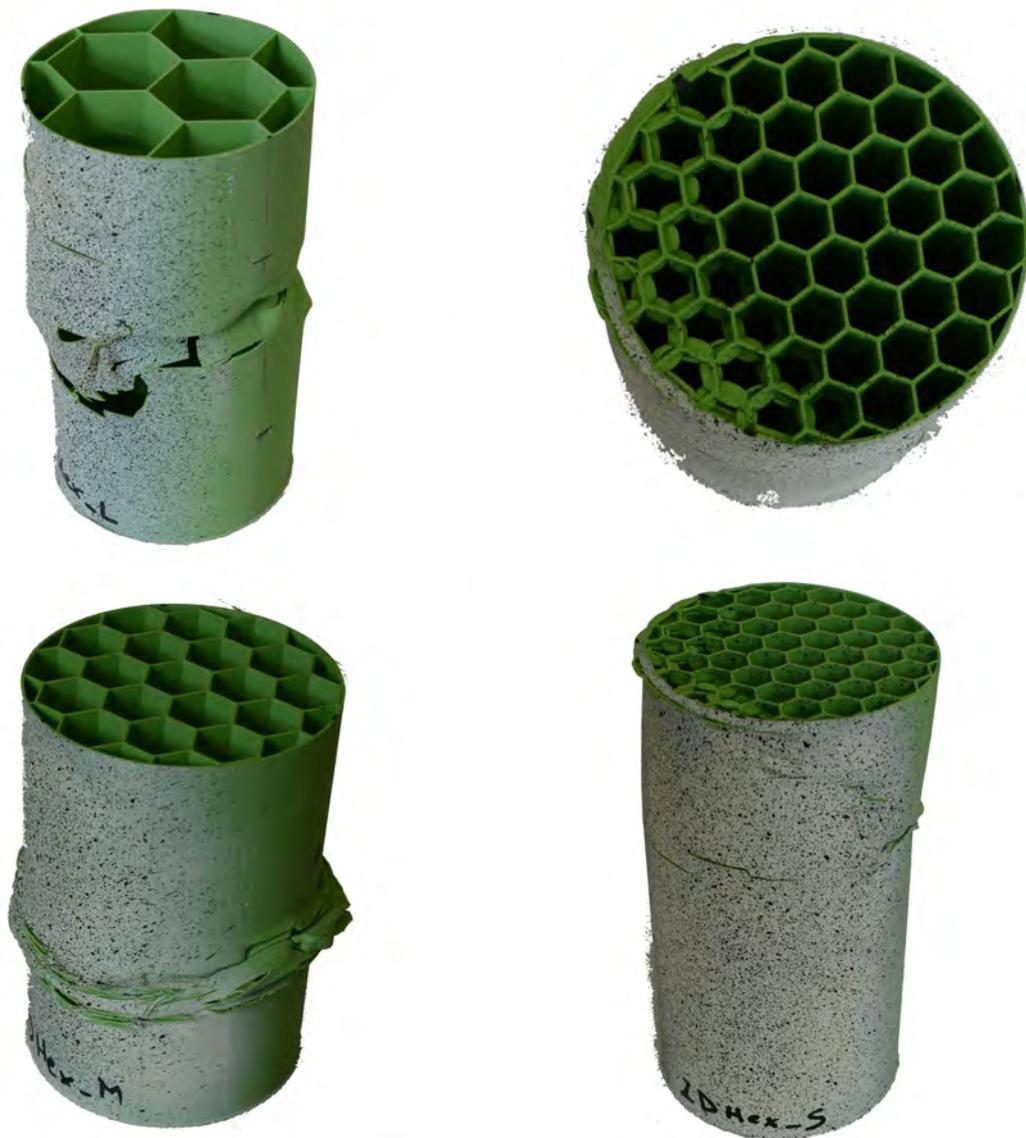
**Figure 9.8:** Sample realizations of cylinder compression tests with 3 scales of reference 2D honeycomb infill. Photographed by the author in 2018.
