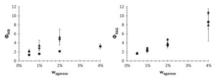
Fig. 3. Partition coefficients of Methylene Blue (left) and Rhodamine 6G (right) in hydrogels with different weight content of agarose at 30 °C ( $\bigcirc$ ), 40 °C ( $\diamondsuit$ ) and 50 °C ( $\triangle$ ).
