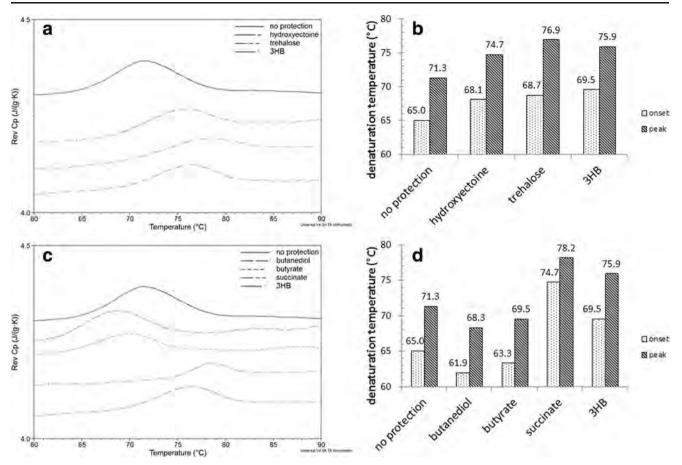
**Fig. 5** DSC signals showing thermal denaturation of lysozyme comparing thermoprotective effect of 3HB, trehalose and hydroxyectoine at 1000 mM (a) and 3HB, 1,3-butanediol, butyrate, and succinate at 1000 mM, respectively (c); *curves* are offset for clarity.
