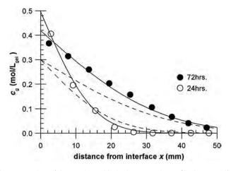
**Fig. 8.** Comparison of the experimental (points) concentration profiles ( $c_0$ =0.6 mol/L) with those calculated for determined diffusion characteristics (solid line) and for diffusion in water (dashed lines).
