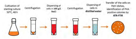
Figure 1: Principle of the "osmoselection"; proceedure enabling isolation of PHA-producing thermophiles:
