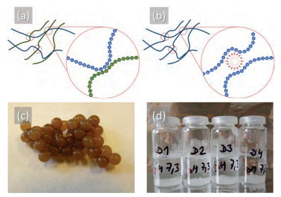
*Fig.* 85 Schematic representation of the electrostatically cross-linked hydrogels under investigation: a) Polyelectrolyte complexes. b) Surfactant-polyelectrolyte hydrogels. Examples of the developed hydrogels: c) Humic acids complexed with chitosan. d) DEAE-SDS hydrogels.
