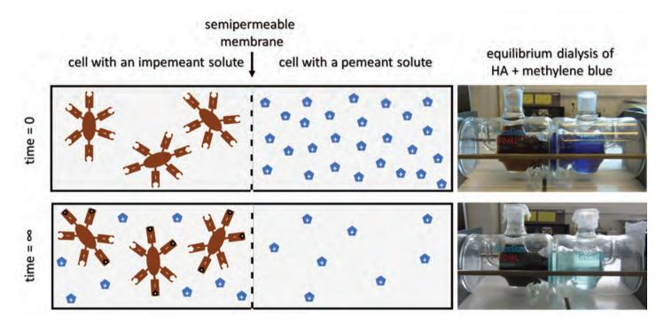
*Fig. 18 Schematic diagram of the solute binding study based on equilibrium dialysis (left). At the start of the experiment, the impermeant binding solute is separated from the permeant solute by an appropriate semi-permeable membrane. The concentration of the permeant solute is monitored until the equilibrium is reached. Images of the experimental apparatus at the start of the experiment (top) and at the equilibrium (bottom) are also shown (right).*
