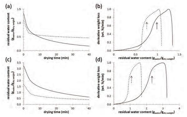
Fig. 54 Results of isothermal thermogravimetry determination of intracellular water content. Raw thermograms (a, c) and drying rate profiles (b, d) of PHA containing cultures of C. necator H16 (a, b) and non-accumulating mutant C. necator  $PHB^{-4}$  in control isotonic buffer (solid line) and in 200 g/L NaCl (dashed line).
