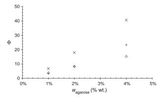
Fig. 5. Partition coefficient for the methylene blue partitioning at the boundary of agarose hydrogels at 25 °C (×), 40 °C (+) and 50 °C ( $\diamond$ ).
