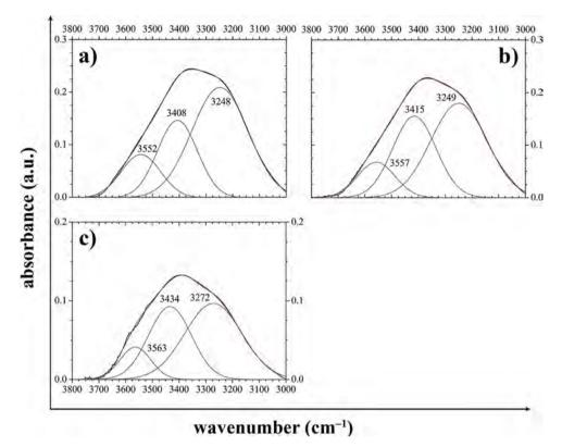
Fig. 7. Example of deconvolution of O-H stretching band for D1 hydrogel at time 0 (a), 60 (b) and 360 min (c), respectively.
