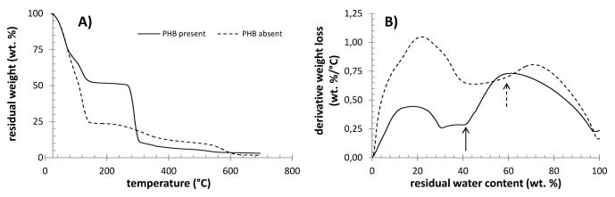
Fig 6. Results of dynamic TGA analysis of centrifuged PHB-containing and PHB non-containing cultures of *C. necator*. A) Weight loss at a heating rate of 10°C/min in the interval 25–700°C, B) derivative weight loss as a function of residual water content (arrows indicate critical water content).
