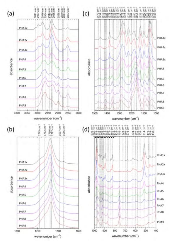
**Figure 1.** Normalized ATR FTIR spectra (cut-offs for the analytically important spectral regions) of the solution-casted PHA films prepared from polymers with different monomer composition (each spectrum represents an arithmetic average of 10 individual spectra collected at different locations on the surface of the film). Frequencies of the absorption band maxima were determined from the second derivative of the spectra.
