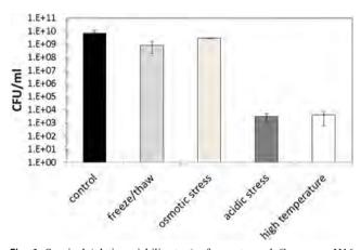
**Fig. 6** Survival (plating viability test) of non-stressed *C. necator* H16 cells (control) and of the cells exposed to different stress factors. (freeze/thaw: culture exposed to 4 cycles of freezing and thawing; osmotic stress: culture incubated in 200 g/L NaCl solution; acidic stress: culture incubated at pH = 1; high temperature: culture incubated at 80 °C). Errors bars represent standard deviation of the 5 parallel samples
