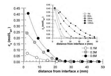
**Fig. 4.** Concentration profiles of Cu<sup>2+</sup> in gel samples (time-variable source) for different initial concentrations of solution (larger figure; example for time duration 24 h) and for various times (smaller figure; example for initial concentration of solution 0.6 mol/L).
