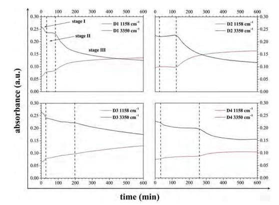
Fig. 6. Time dependences of absorbances at frequencies characteristic for water (-OH at 3350 cm<sup>-1</sup>) and for dry matter content (glycosidic bond at 1158 cm<sup>-1</sup>), respectively, during the FTIR-assisted drying of the gels.
