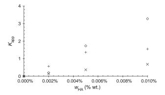
Fig. 9. Apparent equilibrium constant for the sorption of methylene blue in agarose/HA gels at 25 °C (×), 40 °C (+) and 50 °C ( $\diamond$ ).
