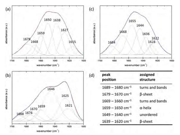
**Fig. 4** Example of deconvolution of Amide I band in *C. necator* H16 (blue: measured spectrum, grey: deconvolution components, red: cummulative fitting spectrum) for (**a**) control sample, (**b**) sample
