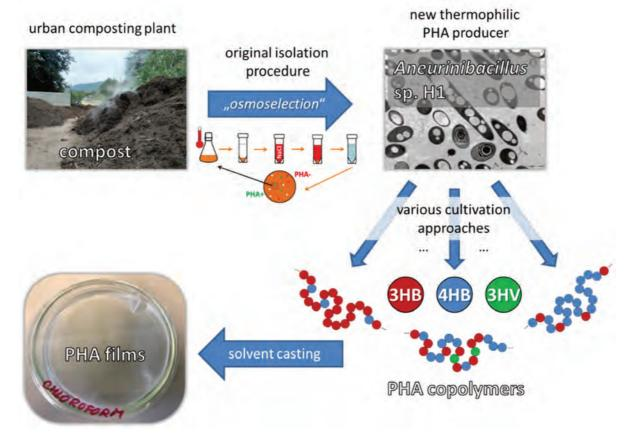
*Fig. 36* Schematic diagram of recently developed strategy for the production of copolymer PHAbased bioplastic films
