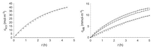
Fig. 3. Breakthrough curves of KCl (left) and MB (right) for diffusion through SPI-Pore membrane. Line represents the theoretical model, scatter plot show the experimental data at 25 °C (×), 40 °C (+) and 50 °C (◊).
