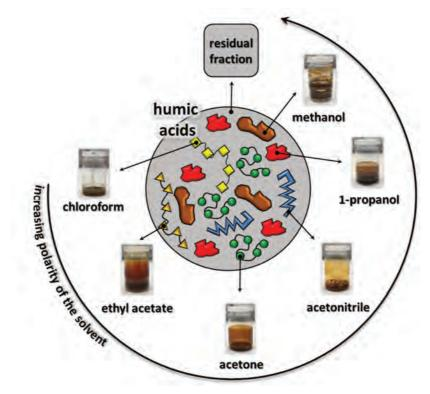
*Fig.* 24 *Schematic diagram of original polarity-based extraction method developed for fractionation of humic acids*
