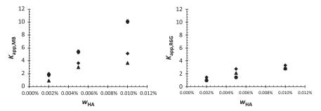
Fig. 7. Apparent equilibrium constants for the diffusion of Methylene Blue (left) and Rhodamine 6G (right) in 1 wt.% agarose hydrogels with different weight content of HA at 30 °C (○), 40 °C (◊) and 50 °C (△).
