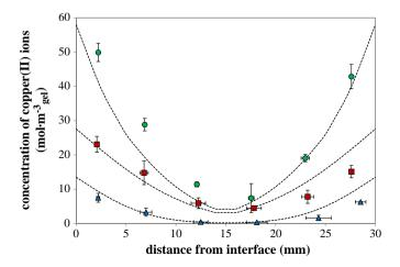
**Fig. 2.** Concentration profiles of diffused copper (II) ions extractable by water ( $\Delta$ ), 1 M MgCl<sub>2</sub> ( $\Box$ ), 1 M HCl ( $\bigcirc$ ) after one day. Data fitted by theoretical Eq. (3) (dashed lines).
