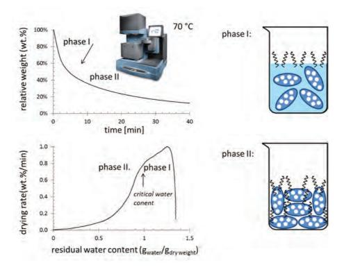
Fig. 53 Schematic representation of the determination of intracellular water content by isothermal thermogravimetry. Effective intracellular water content is determined from the critical point in the drying profile where the steep change in the drying rate appears (marked with an arrow).
