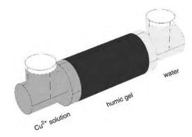
Fig. 1. Scheme of an apparatus for the study of a nonstationary diffusion.
