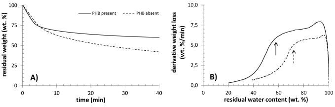
Fig 7. Results of isothermal TGA analysis of centrifuged PHB containing and PHB non-containing cultures of *C. necator*. A) Weight loss at 60°C, B) derivative weight loss as a function of residual water content (arrows indicate critical water content).
