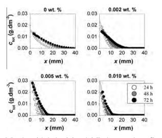
**Fig. 6.** Experimental (points) and theoretical (lines) concentration profiles of Methylene Blue in 1 wt.% agarose gels with the addition of humic acids at 30 °C (the corresponding weight content of HA is shown above each graph).
