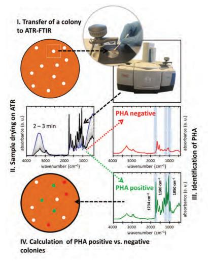
Fig. 68 General experimental procedure for identification of PHA positive and PHA negative colonies by ATR-FTIR as utilized in isolation of thermophilic PHA producers from mixed microbial consortia.
