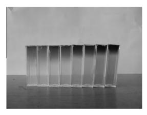
**Fig. 5.** Picture of the gel samples after 24 h of diffusion of Methylene Blue at 30 °C (four duplicates from left to right: 0 wt.%, 0.002 wt.%, 0.005 wt.% and 0.010 wt.% HA in 1 wt.% agarose gel).
