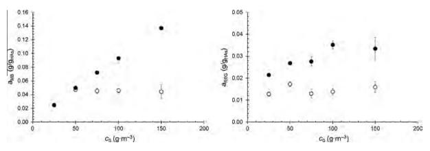
Fig. 4. Specific amount of MB (left) and R6G (right) adsorbed on solid LHAs (O) and MHAs (O) from aqueous solutions with different initial concentrations.
