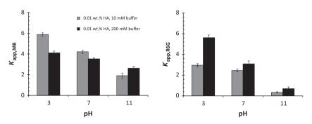
Fig. 9. Apparent equilibrium constants for the diffusion of Methylene Blue (left) and Rhodamine 6G (right) in 1 wt.% agarose hydrogels with 0.01 wt.% of HA at various pH values and ionic strengths at 30 °C.
