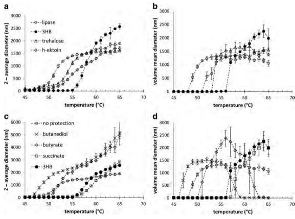
**Fig. 2** Effect of 3HB, trehalose and hydroxyectoine  $(\mathbf{a}, \mathbf{b})$  and 3HB, 1,3butanediol and butyrate  $(\mathbf{c}, \mathbf{d})$  on thermal-induced increase in the particle size of lipase solutions. Studied solutes were applied at 1000 mM
