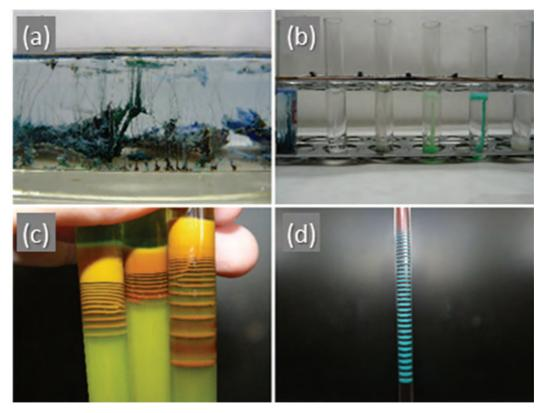
*Fig. 73* Common practical demonstrations of diffusion-related phenomena in hydrogels: chemical gardens (a, b), Liesegang rings (c, d). The procedures used for preparation of the shown phenomena are provided in our paper<sup>XXXVIII</sup>.
