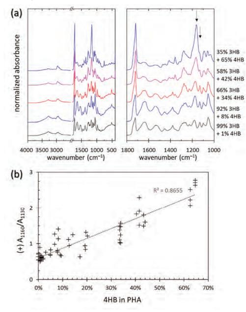
Fig. 43 ATR-FTIR analysis of PHA monomer composition in biomass. (a) ATR FTIR spectra of Aneurinibacillus sp. H1 biomass with accumulated P(3HB-co-4HB) copolymers with various monomer compositions. (b) Correlation of selected FTIR marker of 4HB/3HB content (ratio of absorbances at 1160 and 1130 cm<sup>-1</sup>) with relative content of 4HB in the copolymer (determined for various cultivations including data provided in Fig. 43a).
