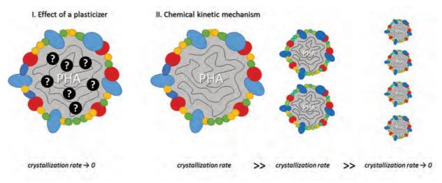
*Fig. 33* Two formerly proposed theories on the mechanism of PHA plasticization in vivo – I. effect of a molecular plasticizer, and II. chemico-kinetic model based on limited volume of the granules.
