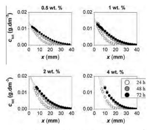
**Fig. 1.** Experimental (points) and theoretical (lines) concentration profiles of Methylene Blue in agarose gels at 30 °C (the corresponding weight content of agarose is shown above each graph).
