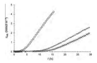
**Fig. 1.** Break-through curves from the diffusion cell experiments. The curves show the concentration of MB in acceptor cell as a function of time for the diffusion through 1 wt.% agarose gel with 0 wt.% HAs  $(\bigcirc)$ , 0.01 wt.% MHAs (+) and 0.01 wt.% LHAs  $(\times)$ .
