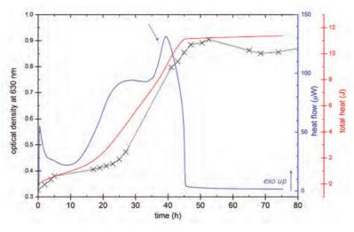
Fig. 60 Monitoring the growth of C. necator H16 culture at 25°C by classical photometric assay (×) and via microcalorimetry (blue and red curves). Results from the microcalorimetric assay are provided as instantaneous heat flow between the sample cell and the heat sink (blue) and as integral heat released from the sample (red). Calorimetry and optical density measurements correspond to two independent cultivations.
