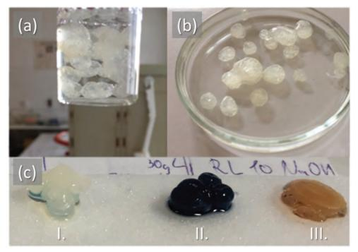
Fig. 86 Hydrogels prepared via cross-linking of chitosan by rhamnolipids. (a,b) Hydrogel beads are prepared by dropwise addition of acidic chitosan into the aqueous solution of rhamnolipids. (c) The ability of the chitosan-rhamnolipid gels (I.) to solubilize hydrophobic compounds as demonstrated for non-polar dyes Sudan black (II.) and Sudan red (III.).
