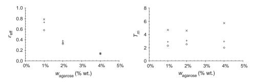
Fig. 6. Calculated effective porosities and tortuosity factors of agarose hydrogels at 25 °C (×), 40 °C (+) and 50 °C (◊).
