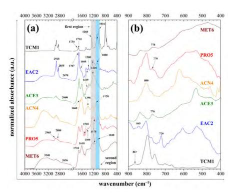
**Figure 1.** Attenuated Total Reflectance (ATR-FTIR) spectra of organic fractions extracted from peat HA, (**a**) spectral range of 4000–400 cm<sup>-1</sup> and (**b**) spectral range of 900–400 cm<sup>-1</sup> for the visualization of less intense absorption bands.
