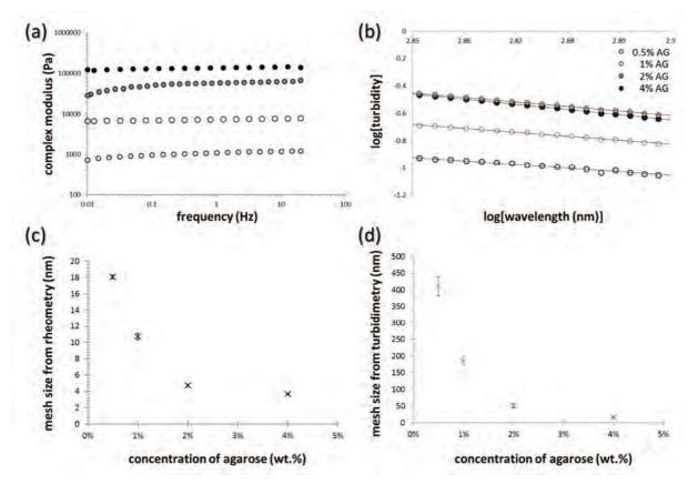
Fig. 78 Indirect determination of pore size of the agarose hydrogels from oscillatory rheometry (a,c) and turbidimetry (b,d). Original data was obtained by the technique (a, b), and calculated mesh sizes were calculated from these data (c,d) as a function of agarose concentration in the gel. Data published in<sup>XL</sup>.
