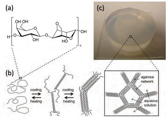
Fig. 74 Agarose hydrogel as a multi-purpose medium for experimental diffusion studies. Molecular structure of agarose (a) and the schematic illustration of the macromolecular aggregation processes (b) which take place during the thermoreversible agarose gelatinization leading to the final agarose hydrogel (c).
