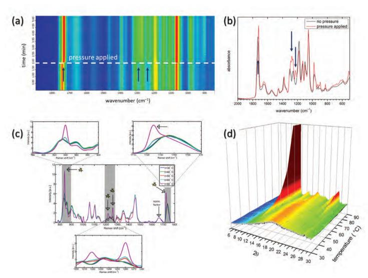
Fig. 44 Monitoring of PHA crystallization in biomass by various methods of structural analysis. PHA crystallization was induced by exposing the dry biomass of C. necator H16 to mechanic pressure (a, b) and radiant heat (c, d). Spectral markers of crystallization as observed in FTIR 2D and 1D spectra, respectively (a, b), Raman spectra (c) and X-ray diffraction spectrum (d).
