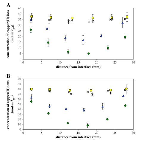
**Fig. 3.** Time development of concentration profiles of diffused copper (II) ions extractable by 1 M MgCl<sub>2</sub> (A) and 1 M HCl (B). The profiles after 1 ( $\bigcirc$ ), 3 ( $\triangle$ ), 7 ( $\times$ ), 11 ( $\diamond$ ) and 20 ( $\square$ ) days are shown.
