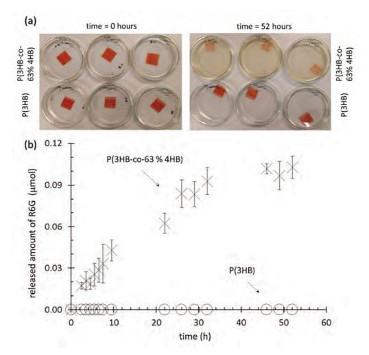
Fig. 38 Example of results from a preliminary study on transport properties of PHA polymers with different monomer composition – release of Rhodamine 6G incorporated into the film during solvent-casting (concentration of R6G in the polymer solution 1g/L). (a) Picture of the samples at the start and the end of the release experiment. (b) Kinetics of R66 release during the first ten hours of the experiment.
