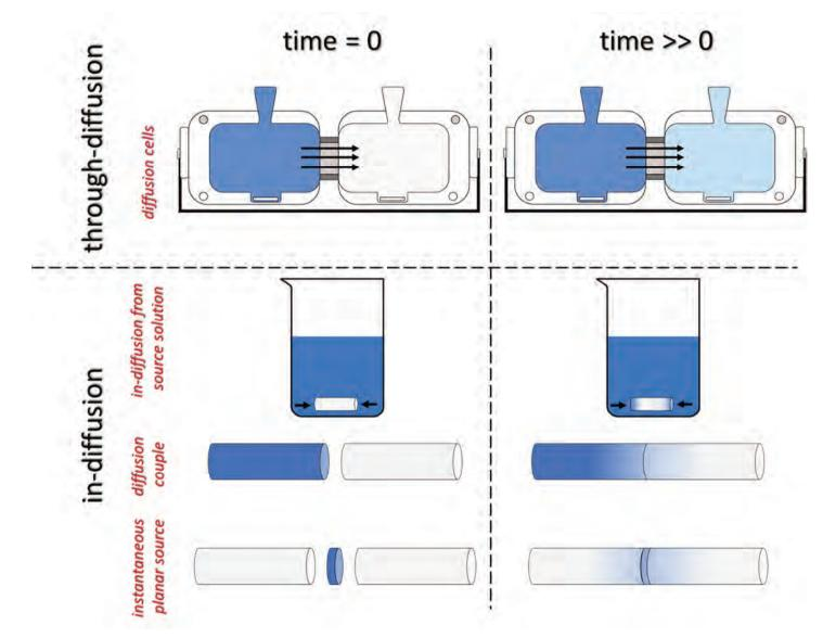
*Fig.* 15 *Various setups used in the developed diffusion methodology*
