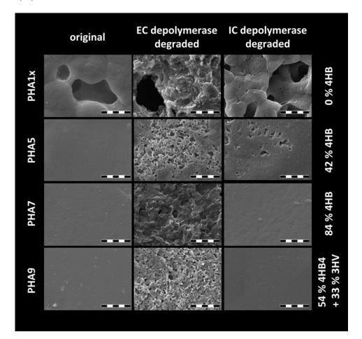
Figure 7: SEM micrographs of PHA complymentifilms before and after the enzymatic degradation assay exingenting (EC) of 1 AC de BHAm degely merase and in the physical action of the second s respectively (magnification 10,000 scale bar: 10 µm).
