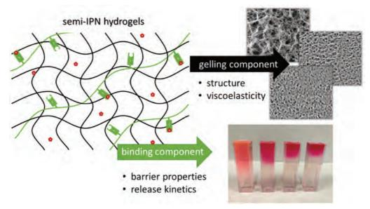
Fig. 82 Proposed strategy of tailoring performance and properties of semi-IPN hydrogels. An inert gel-forming polymer network is interpenetrated by a linear polymer component with the properly selected binding functionality. Mechanical and transport performance of the material is adjusted independently via manipulating the relative content of the two structural components.
