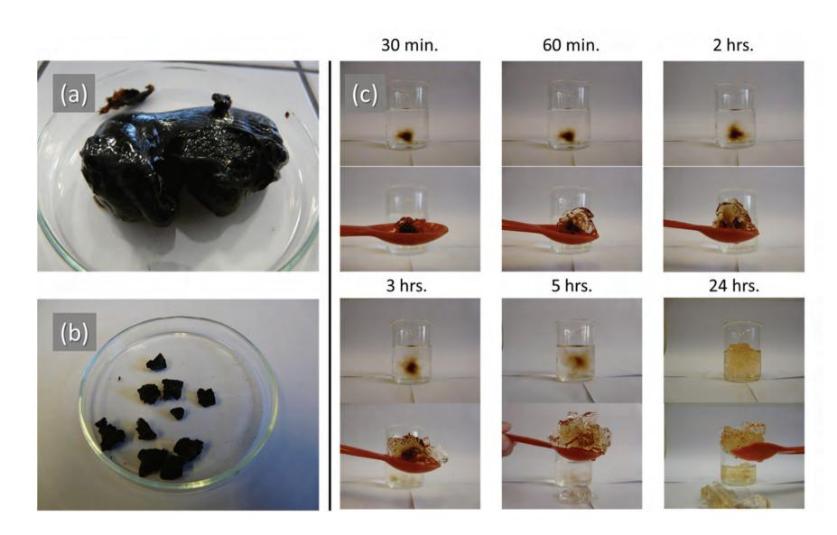
*Fig.* 84 Superabsorbent polymer (SAP) material based on polyacrylate chains grafted on humic substances. Polymerized SAP as-prepared (a) and in the dried form (b). Monitoring the swelling of the SAP in deionized water (c).
