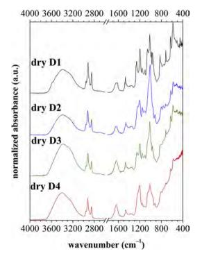
**Fig. 3.** ATR-FTIR spectra of all tested dry polyelectrolyte-surfactant hydrogels. DEAE-dextran gels with SDS (black and blue solid curve) and DEAE-dextran gels with linear STS (green and red solid curve) (For interpretation of the references to colour in this figure legend, the reader is referred to the web version of this article).
