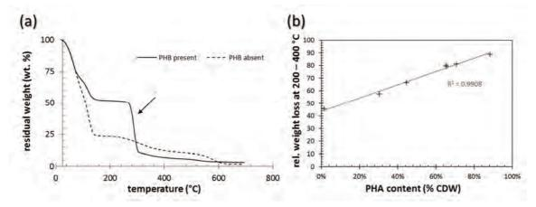
Fig. 40 Thermogravimetry of PHA producing cells (heating rate: 10°C/min, atmosphere: air). (a) Thermogram showing the temperature range at which PHA degradation is manifested (marked with arrow). (b) Correlation between relative weight loss in the range from 200 to 400 °C and the weight content of PHA.
