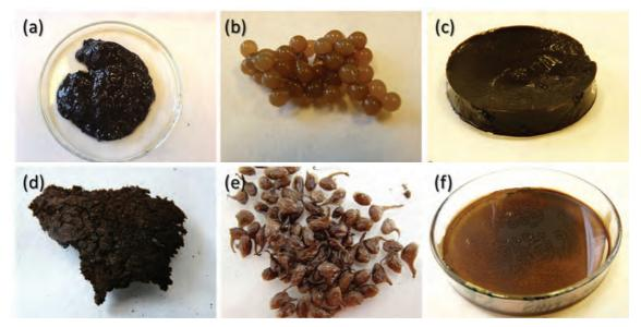
Fig. 28 Swelled (a-c) and the corresponding dried (d-f) forms of HA-chitosan hydrogels. (a,d) Macrogel prepared by fusion of chitosan and HA solutions. (b,e) Hydrogel beads prepared by adding a viscous chitosan solution dropwise into HA solution. (c, f) Whole-volume gelation via alkalization of chitosan/HA mixture by ammonia vapors. Drying of the gel (c) results in film (f) with a high swelling ability.
