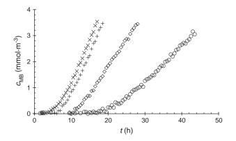
**Fig. 8.** Breakthrough curves of MB for the diffusion at 25 °C through 1 wt.% agarose hydrogels with 0 wt.% ( $\times$ ), 0.002 wt.% (+), 0.005 wt.% ( $\diamond$ ) and 0.010 wt.% ( $\bigcirc$ ) of HA.
