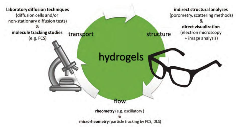
*Fig.* 75 *Schematic representation of the developed methodology for multiscale experimental study on the relationships between internal structure, mechanical (flow) properties, and transport or barrier properties of hydrogels under investigation.*
