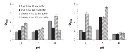
Fig. 10. Partition coefficients for the diffusion of Methylene Blue (left) and Rhodamine 6G (right) in 1 wt.% agarose hydrogels with 0.01 wt.% of HA at various pH values and ionic strengths at 30 °C.
