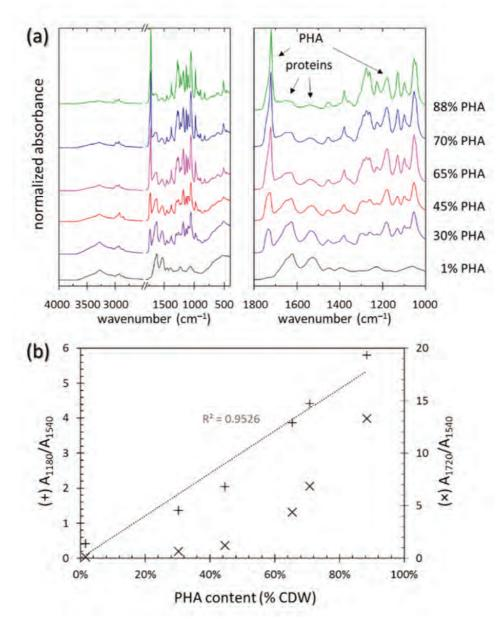
Fig. 42 Semi-quantitative analysis of PHA in biomass by ATR-FTIR spectroscopy. (a) ATR spectra of dry biomass of C. necator H16 with different amounts of accumulated PHA (determined by GC-FID). (b) Correlation of selected FTIR markers of PHA (absorbances at 1720 and 1180 cm<sup>-1</sup>, respectively, normalized on amide II band at 1540 cm<sup>-1</sup>) with PHA content in biomass.
