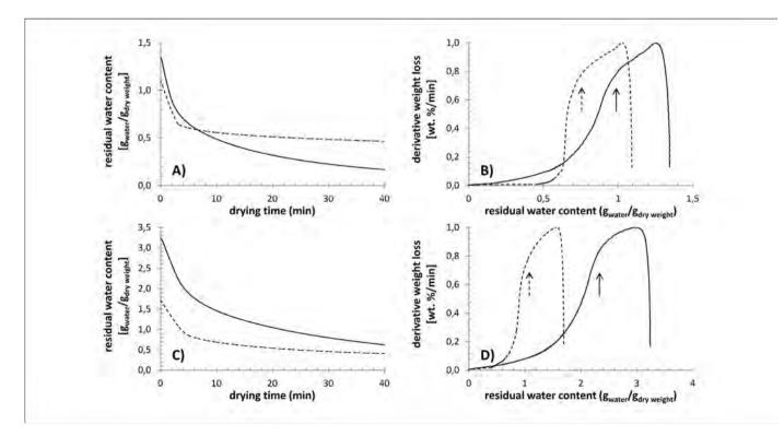
Fig. 7. The effect of osmotic challenge on drying curves determined by isothermal TGA experiments at 60 °C on *C. necator* H16 (A, B) and *C. necator* PHB-4 (C, D). Solid lines represent unchallenged bacterial samples, dashed lines represent samples exposed to 200 g/L NaCl. The heights of the derivative weight loss curves (B, D) were normalized for clarity. Arrows indicate respective critical water contents.
