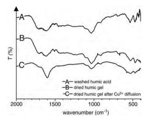
Fig. 9. Transmittance FT-IR spectra of used HAs (A), humic gel (B) and humic gel with diffused  $Cu^{2+}$  ions (C).
