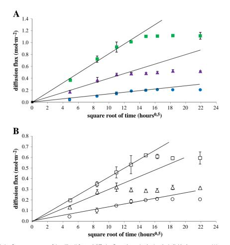
Fig. 4. The dependence of diffusion flux on square root of time (Eq. 4) for total diffusion fluxes determined using the individual extractants (A): water (●), 1 M MgCl<sub>2</sub> (▲), 1 M HCl (■); and for diffusion fluxes computed for the individual copper(II) fractions (B): mobile (○), ion-exchangeable (△), strongly bound (□). Linear parts of the dependences are fitted with lines.
