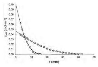
**Fig. 2.** Concentration profiles of methylene blue in 1 wt.% agarose gels with 0 wt.% LHAs  $(\bigcirc)$  and 0.01 wt.% LHAs  $(\times)$  after 72 h of the in-diffusion experiment.
