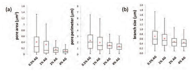
*Fig.* 81 *Results of structural analysis of agarose gels provided by processing cryoSEM images using Particle analysis (a) and Skeleton analysis (b) in ImageJ.*
