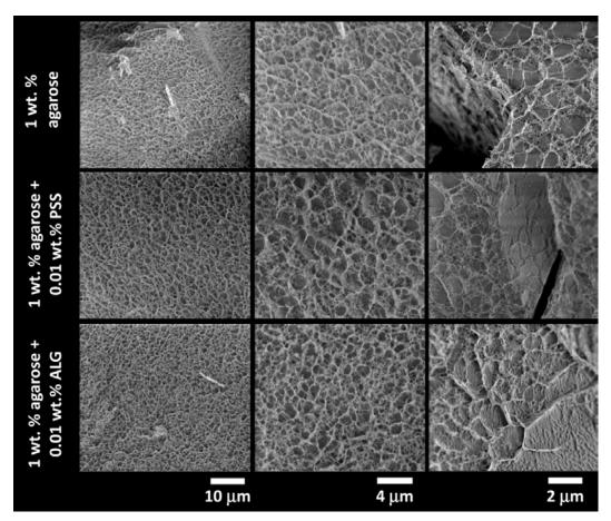
Figure 5. Results of cryo-SEM imaging of the internal structure of the plunge-frozen 1wt.% agarose Figure 5. Results of cryo-SEM imaging of the internal structure of the plunge-frozen 1wt.% agarose hydrogels with and without the presence of an interpenetrating polyelectrolyte component (0.01 wt.% hydrogels with and without the presence of an interpenetrating polyelectrolyte component (0.01 wt.% of PSS and ALG, respectively).
