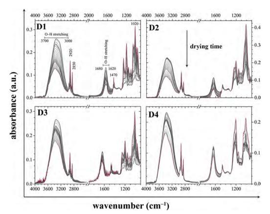
Fig. 4. Development over time of the ATR-FTIR spectra of tested polyelectrolyte-surfactant hydrogels.
