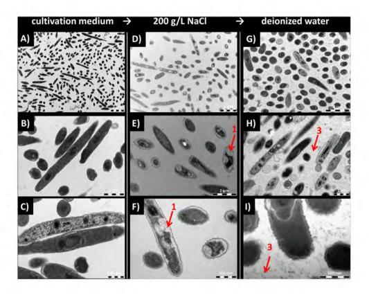
**Fig. 4.** TEM micrographs of *C. necator* PHB-4 observed under different magnifications after cultivation in mineral medium (A – C), after hyperosmotic treatment in 200 g/L NaCl (D–F) and after additional hypoosmotic treatment in deionized water (G–I). Severe plasmolysis (1) and leakage of the cytoplasmatic content (3) is labeled in the pictures.
