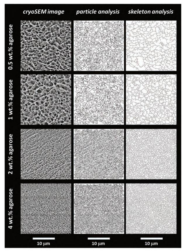
*Fig. 80* Determination of pore size of the agarose hydrogels via analysis of cryoSEM images using two image processing tools implemented in ImageJ (Skeleton analysis and Particle analysis).
