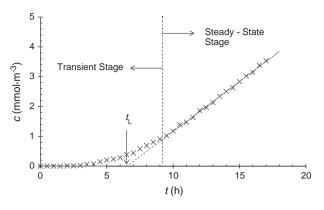
Fig. 2. Concentration of the solute in acceptor compartment as function of time (1 wt.% agarose hydrogel, 25  $^{\circ}$ C).
