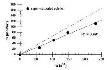
Fig. 3. Dependence of the total diffusion flux on the square root of time (constant source) as compared with the flux calculated for diffusion in water (dashed line).
