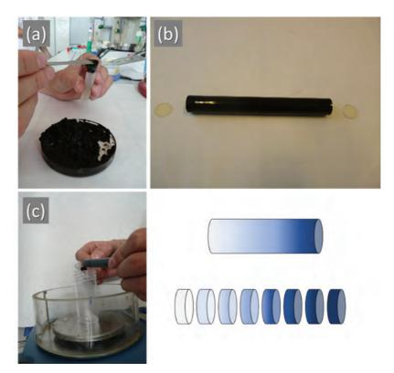
Fig. 16 The main experimental steps in diffusion studies on the humic acid gels. (a) Filling the gel into the tube carrier. (b) Diffusion experiment (in diffusion couple on the picture). (c) Slicing the gel in order to determine the concentration profile of the diffusing solute.
