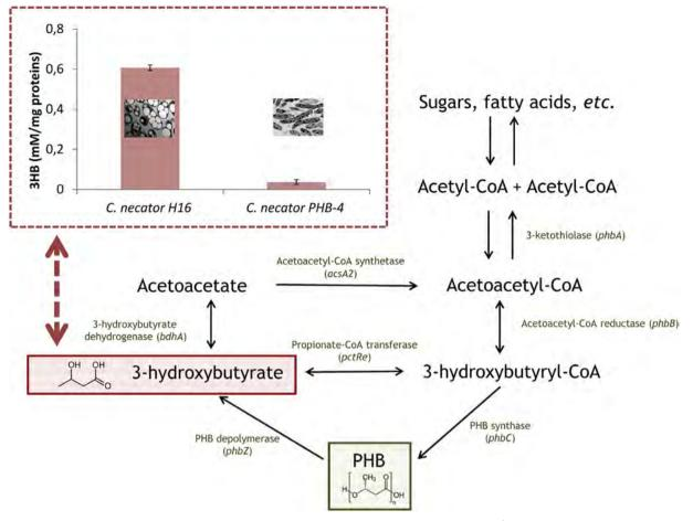
Fig. 2. Difference in 3HB content in PHB accumulating *C. necator* H16 and its PHB non-accumulating mutant *C. necator* PHB<sup>-4</sup> as a consequence of fully functional PHB metabolic metabolism called PHB cycle. The mutant strain is not capable of PHB biosynthesis due to mutation of *phbC* gene encoding for PHB synthase; hence, the PHB cycle is interrupted and dysfunctional (Obruca et al., 2016c).
