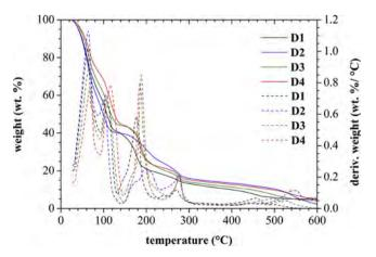
**Fig. 1.** TGA thermograms provided as time evolution of relative weight (solid curves) and the rate of the weight loss (dashed curves) during heating of tested hydrogels in air (heating rate 10 °C/min). Analyzed gels are labeled according to Table 1.
