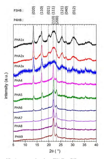
Figure 2. X-ray diffraction patterns of copolymer PHA films. Biffractograms were normalized for clarity. Reflections are assigned to PG(BPB) and P(BPB) that there is pespecial very, according to Caol et al. [25]. and Kertection et al. [27].
