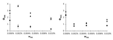
Fig. 8. Partition coefficients for the diffusion of Methylene Blue (left) and Rhodamine 6G (right) in 1 wt.% agarose hydrogels with different weight content of HA at 30 °C ( $\bigcirc$ ), 40 °C ( $\diamondsuit$ ) and 50 °C (△).
