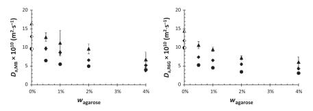
**Fig. 2.** Apparent diffusion coefficients of Methylene Blue (left) and Rhodamine 6G (right) in hydrogels with different weight content of agarose at 30 °C (○), 40 °C (◊) and 50 °C (△). Half – filled points represent the free solution diffusion coefficients.
