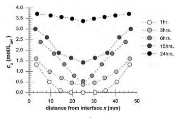
Fig. 2. Concentration profiles of Cu<sup>2+</sup> in gel samples (constant source).
