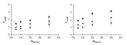
Fig. 4. Tortuosity factors for the diffusion of Methylene Blue (left) and Rhodamine 6G (right) in hydrogels with different weight content of agarose at 30 °C (○), 40 °C (◊) and 50 °C (△).
