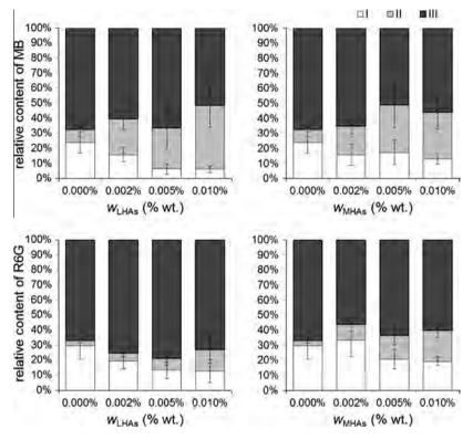
Fig. 3. Distribution of the equilibrium content of the solute in hydrogels into three fractions according to the binding strength: water extractable (I), HCI-extractable (II) and residual (III).
