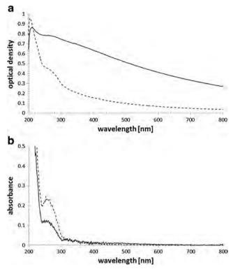
**Fig. 2** Example of typical UV-Vis spectra of *C. necator* H16 (full line) and *C. necator* PHB<sup>-4</sup> (dashed line). **a** Turbidity measurement of dispersions with cell density  $1 \times 10^{6}$  CFU. **b** Absorbance measurement of dispersions with cell density  $1 \times 10^{6}$  CFU
