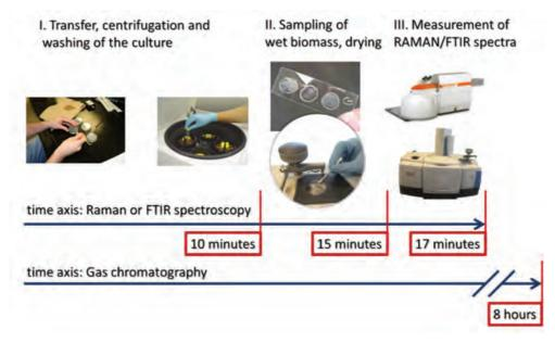
Fig. 41 Timeline showing a reduced time demands on the determination of PHA content in biomass by means of vibrational spectroscopy (Raman or FTIR) as compared to commonly used GC analysis (adopted with modifications from our published study<sup>XIX</sup>).
