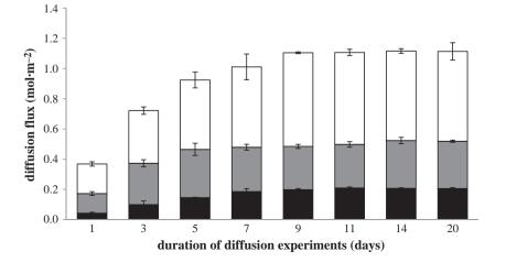
Fig. 6. The time dependence of diffusion fluxes of the individual copper(II) fractions: mobile (black), ion-exchangeable (gray), strongly bound (white).
